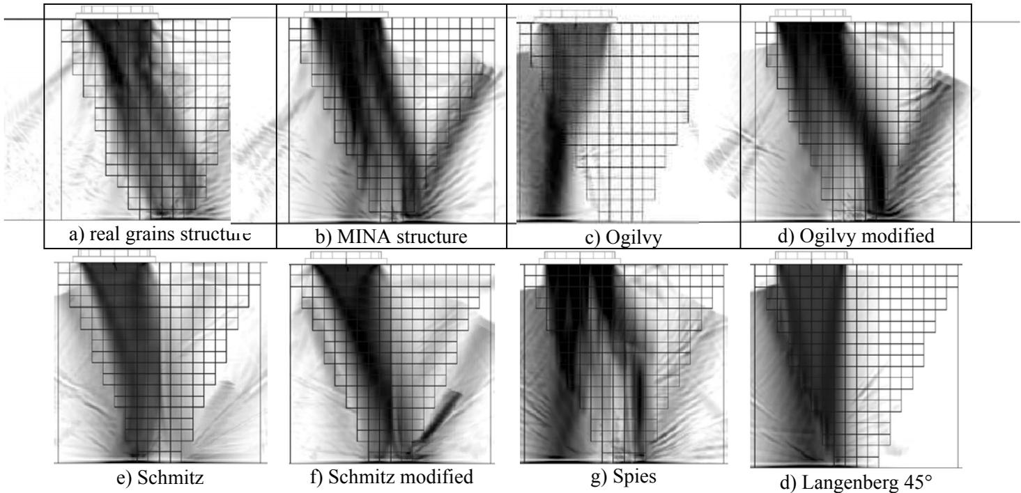
Figure 4. Resulting ultrasonic wave propagation simulated with ATHENA code in simulated grains structure.
