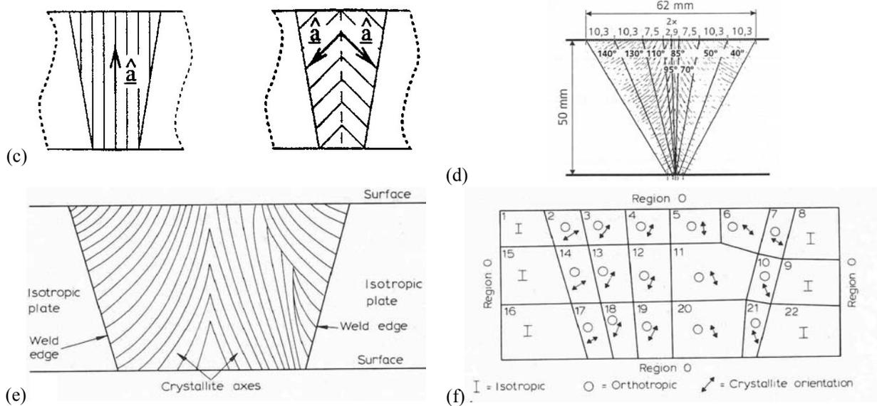
Figure 1. Grains modelling : (a) and (b) used by Ogilvy, (c) used by Langenberg, (d) by Spies (e) and (f) by Silk.
