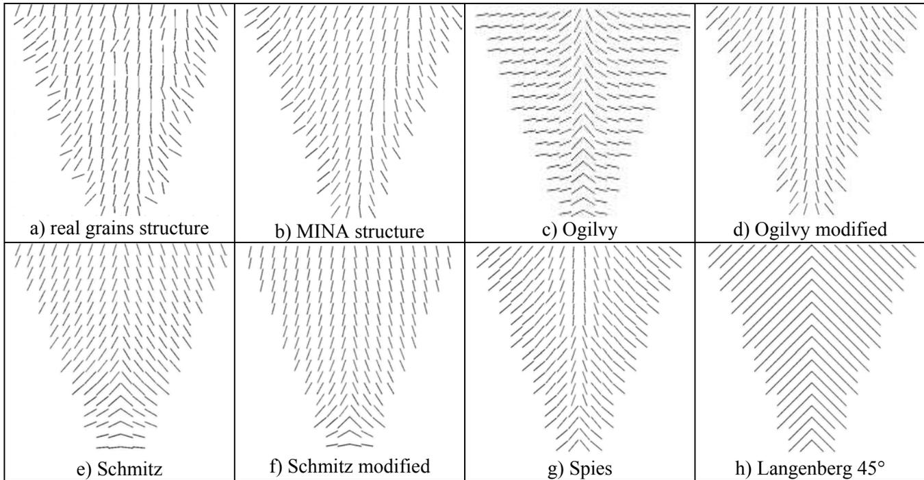
Figure 3. Resulting grains structure for several modelling techniques
