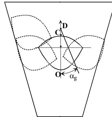
b) schematic representation of multipass welding
