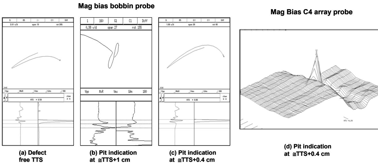
**Figure 8: CTR1 probe impedance display from TTS location in a section of Monel 400 tubing with a pit-like indication, compared CTR2-C4 probe C-scan display.**
