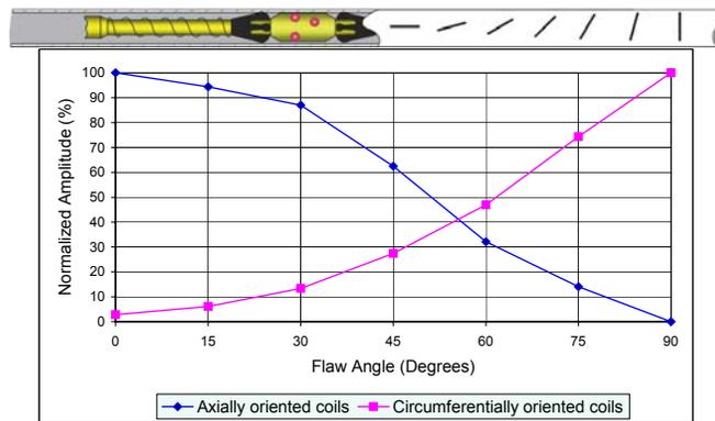
Figure 3: Effect of flaw angle on T/R coil detection capabilities
