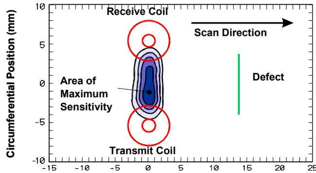
Figure 2: Computer simulation illustrating areas of sensitivity and directional properties of T/R probes
