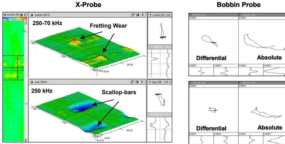
**Figure 6: X-Probe signals from edge fretting-wear under scallop-bars in Incoloy 800 tubing compared to bobbin probe signals. These flaws are sized using a calibration curve based on the 250-70 kHz axial mix channel.**
