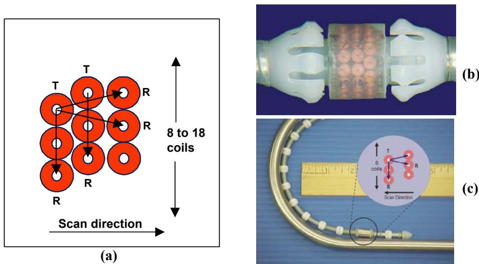
**Figure 5: X-probe for axial and circumferential crack detection (a) coil configuration (b) View of an X- probe for 22.3 mm diameter tubing (c) View of an X-probe for 12.9 mm diameter tight radius U-bend tubing**
