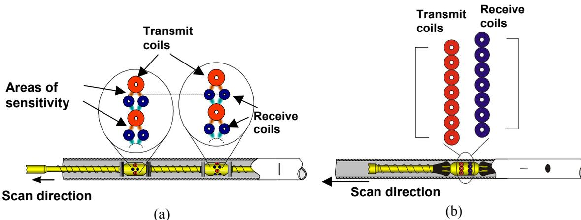
Figure 4: (a) C3 probe for circumferential crack detection showing coil configuration and areas of sensitivity. (b) C4 probe for axial crack detection showing coil configuration.
