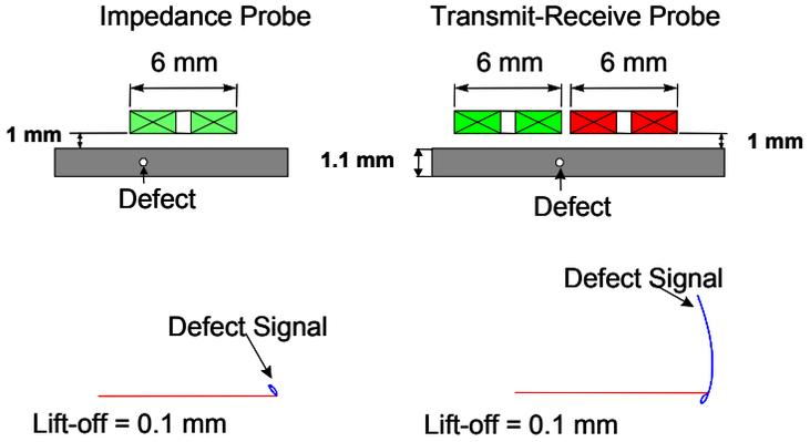
**Figure 1: Comparison of signal-to noise ratio for an impedance probe versus a T/R probe**
