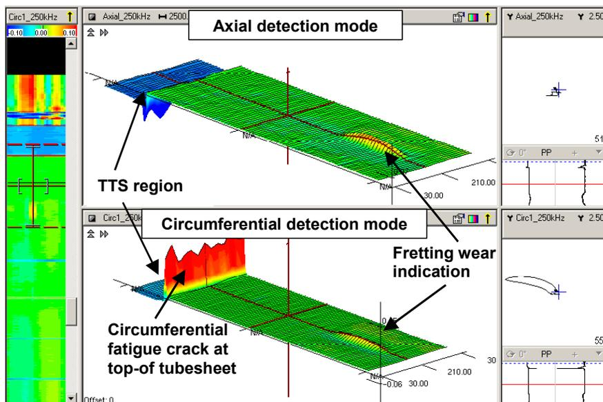
**Figure 7: Array probe helps in assessing degradation mechanism. Example of X-probe signals from an Incoloy 800 tube with fatigue cracking induced by excessive tube vibration.**
