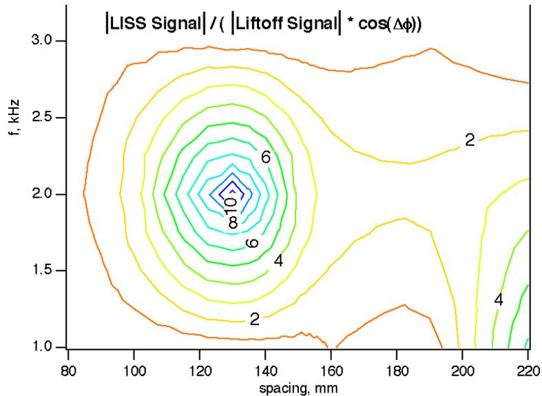
Figure 4: Contour Plot of Performance Factor, Standard Transmit Coil
