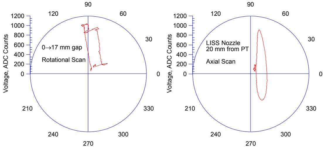
Figure 7: *Lissajous Plots for Response to Gap and LISS Nozzle*
