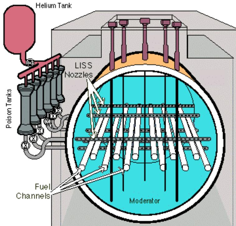
Figure 1: Basic CANDU® Configuration (Only 12 of 380 Fuel Channels Shown)
