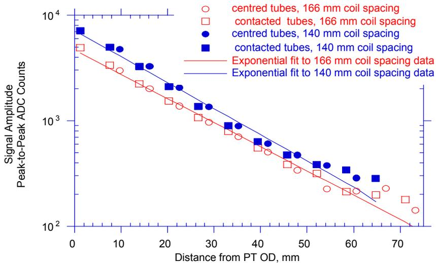
Figure 6: *RFEC Amplitude versus Distance from LISS Nozzle to PT OD*
