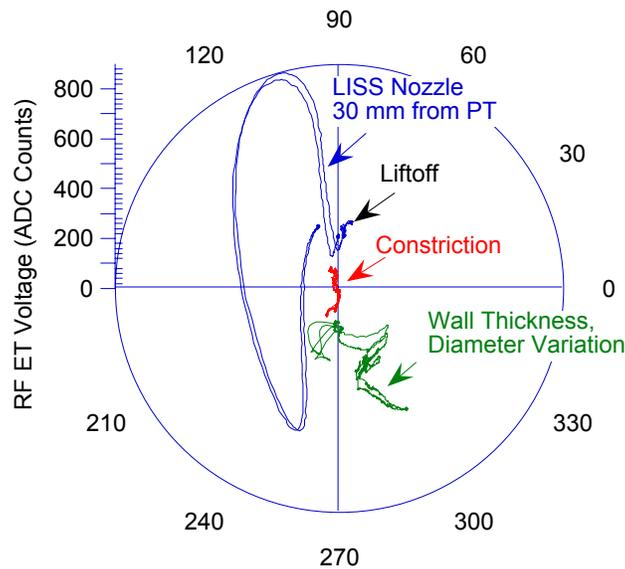
Figure 9: *Lissajous Plots of Signal from LISS Nozzle and Various Noise Sources*
