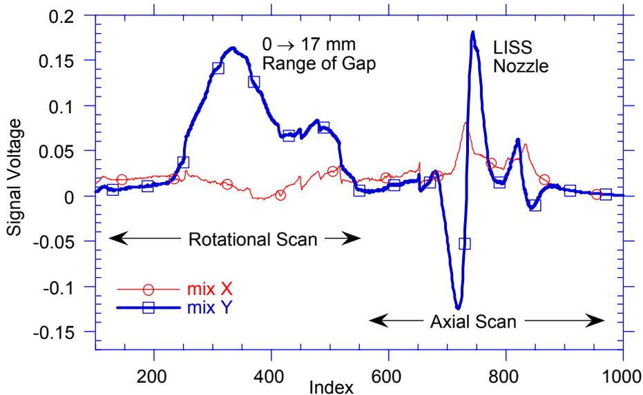
Figure 8: *Gap and LISS Signals, Time-Based Acquisition*
