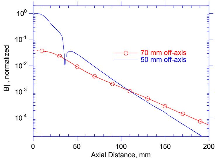
Figure 5: *Magnetic Flux Density Inside and Outside of PT/CT, Focused Transmit Coil*
