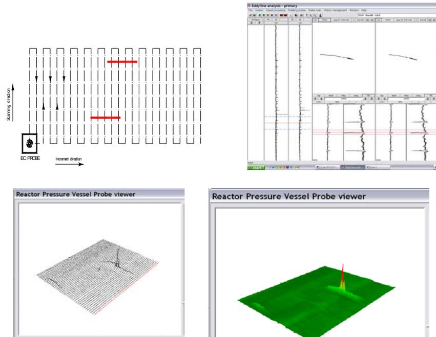
Figure 5 Efficiency of C-scan presentation on specimen with two flaws
