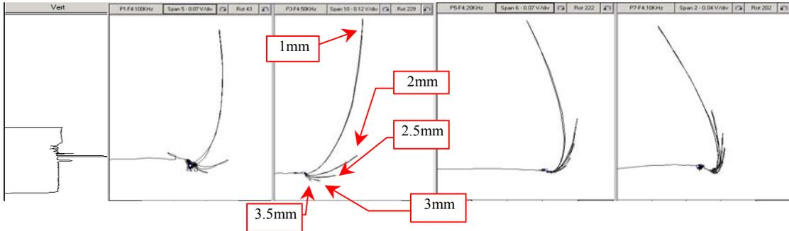
Figure 3. Resolution of subsurface flaws on different frequencies
