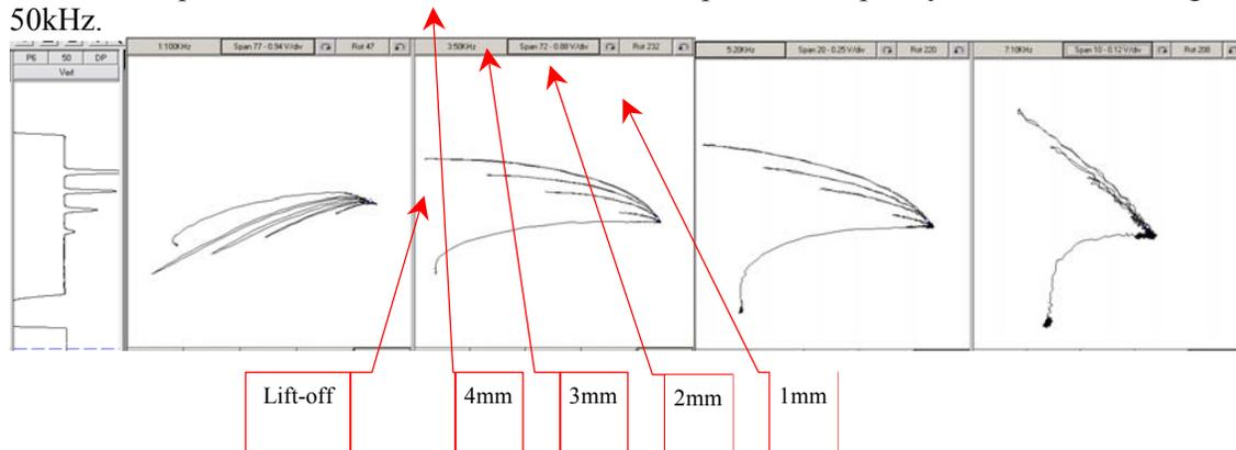
Figure 2. Resolution of surface flaws on different frequencies
