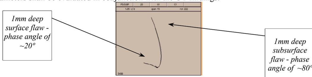
Figure 4. Phase angles of surface and subsurface flaws on 20kHz
