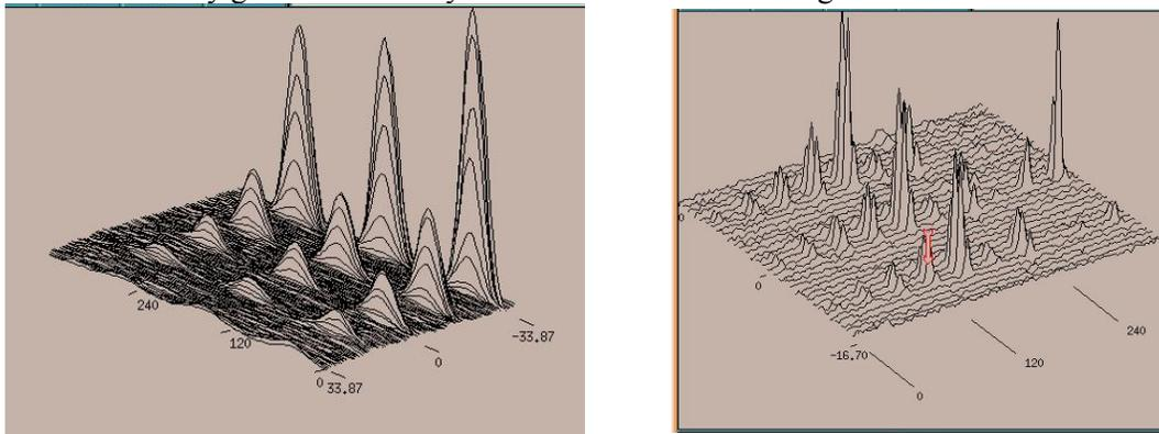
Figure 6. C-scans of scanning same specimen in two orthogonal directions
