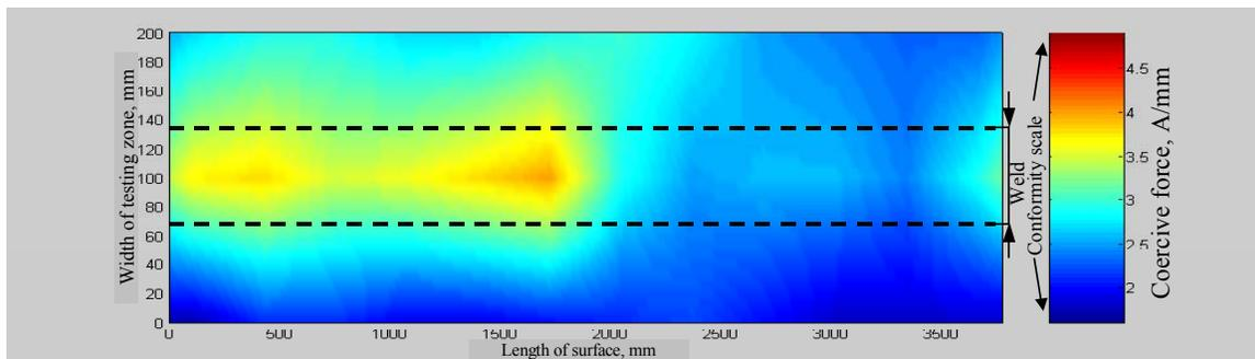
B - new steam generator, from storehouse, has weld anomalies, which can become the future zones of accelerated destruction.
