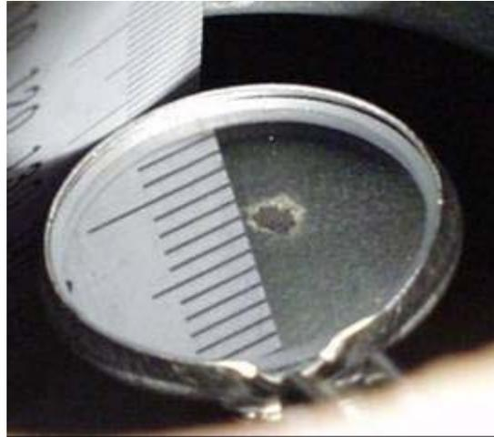
Figure 2. Chip in throat of PRCS thruster.
