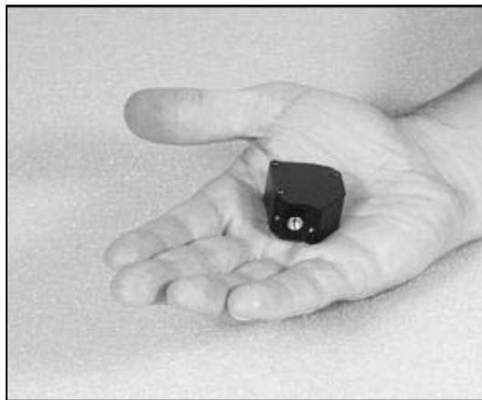
Figure 3. Miniature laser profile sensor developed for NASA
