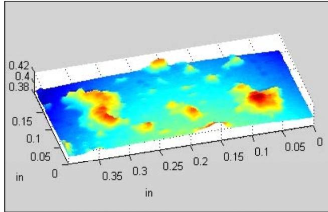
Figure 5. Laser-generated profile of corrosion on a surface.
