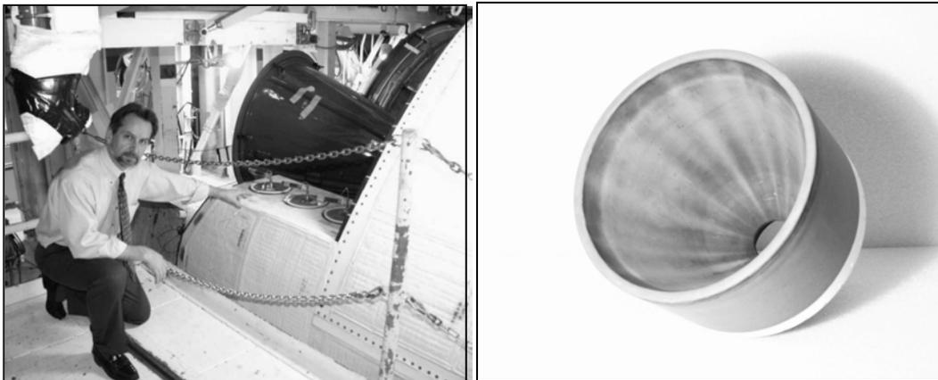
Figure 1. The Space Shuttle has 38 PRCS thrusters located around the orbiter.
