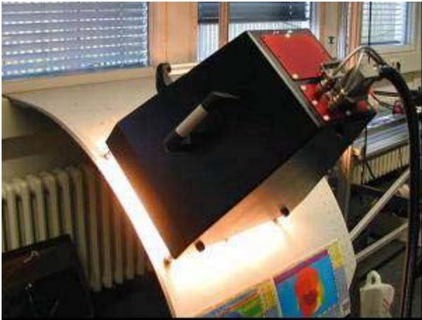
Fig. 5: Performed test on fuselage part of monolithic-CFRP-structure
