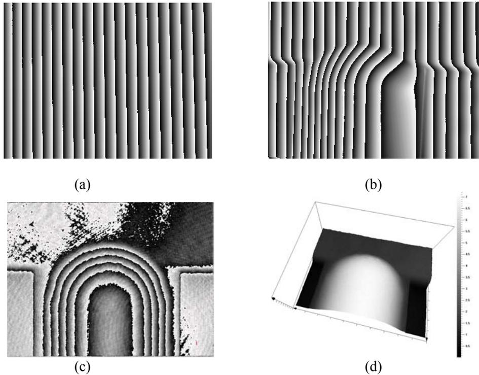
Fig. 3 Principle of 3D-digitization for whole field 3D-shape measurement (a)  $\Delta_f$  of a flat surface (reference plane), (b)  $\Delta_c$  on 3D-object, (c) the phase difference  $\Delta_f - \Delta_c$  and (d) display of 3D-shape [including an operation of  $(\Delta_f - \Delta_c)/K(x,y)$ ]
