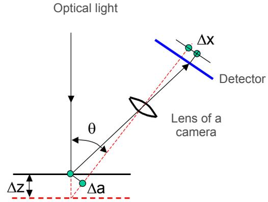
Fig. 1 Principle of Spot of light triangulation
