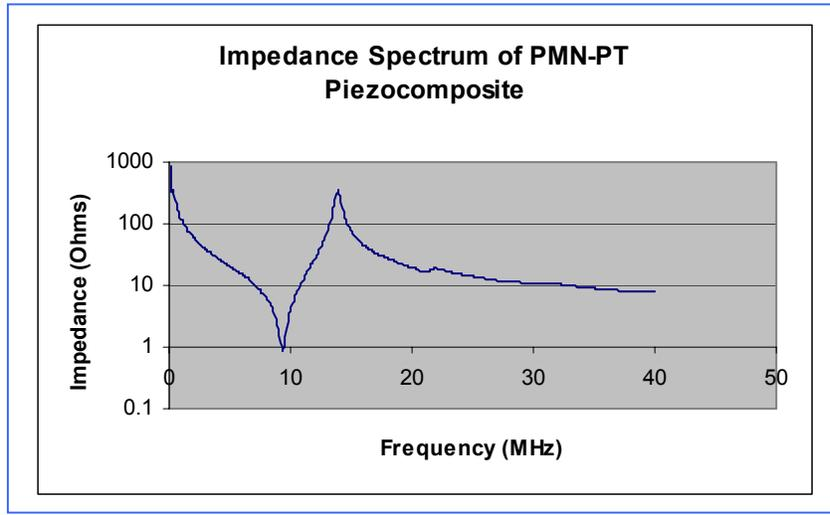
Fig. 6 – Impedance Spectrum of 9.3 MHz PMN-PT Piezocomposite
