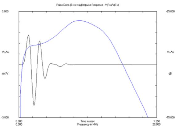
Figure 3 – Pulse-echo Impulse Response of a PZT Piezocomposite Transducer
