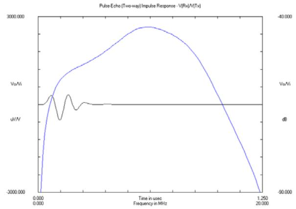
Figure 2 – Pulse-echo Impulse Response of a Lead Metaniobate Transducer
