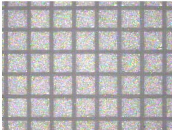
Figure 5 – 60% volume fraction PMN-PT piezocomposite using slower dicing speeds
