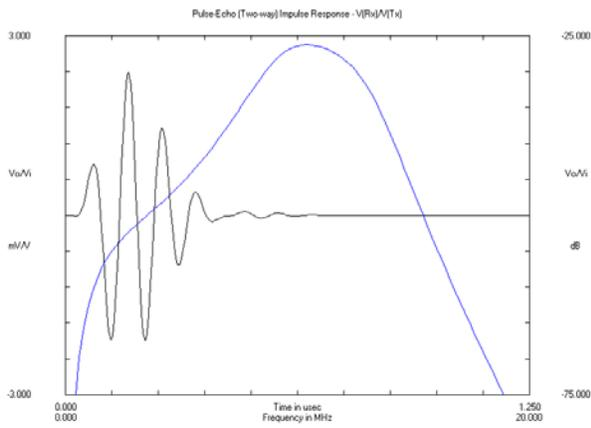
Figure 1 – Pulse-echo Impulse Response of a PZT Transducer
