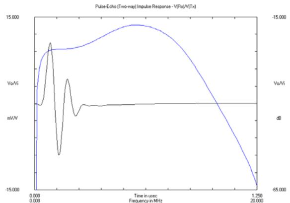
Figure 4 – Pulse-echo Impulse Response of a Single-crystal PMN-PT Piezocomposite Transducer
