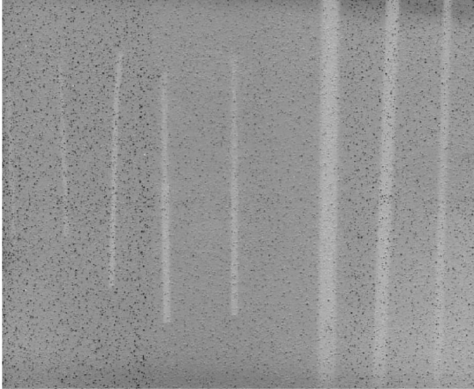
Figure 3: Radiograph of a sediment sample with 4 drill bits (left) and 3 aluminum wires (right).
