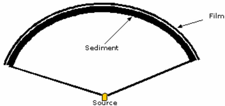
Figure 2: Source-object-film arrangement.
