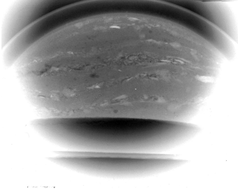
Figure 6: Radiograph of a sediment sample with a fine laminar structure.
