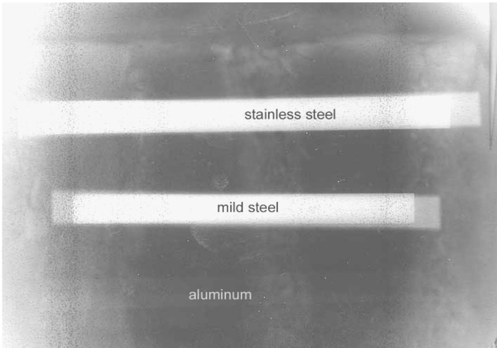
Figure 4: Radiograph of a sediment sample with three different metallic strips.
