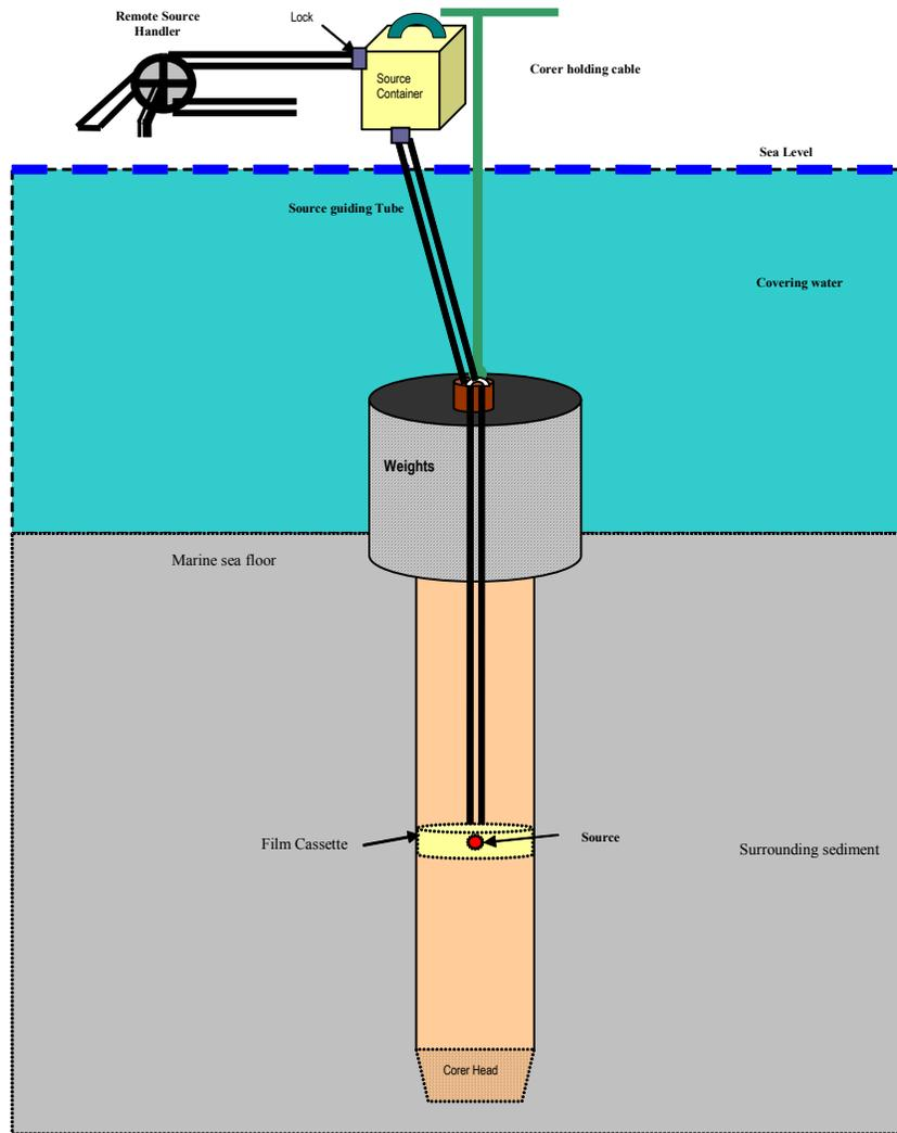
Figure 1: Schematic diagram of a conceived *in situ* radiographic system.
