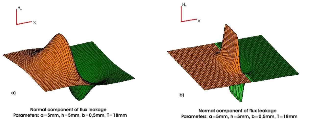
**Fig. 1. Distribution of normal component over external (a) and internal (b) defects.**
