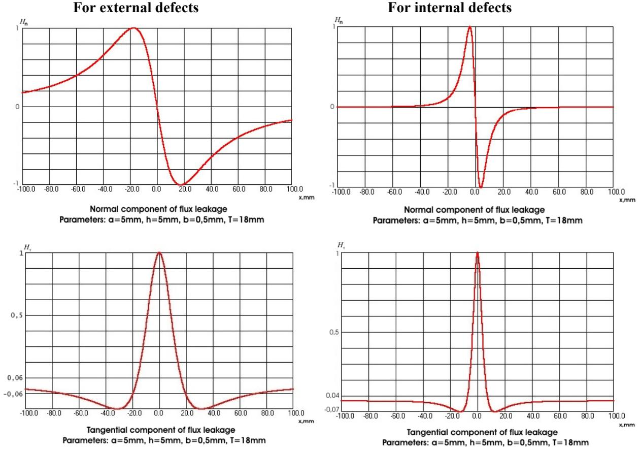
**Fig. 3. Distribution in the direction perpendicular to the pipe axis and in the middle of the crack**
