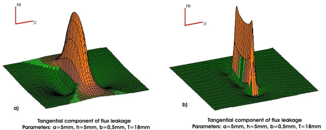
**Fig. 2. Distribution of tangential component over external (a) and internal (b) defects.**
