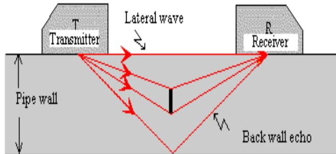
Fig. 3 Transmitter-Receiver arrangement of TOFD <sup>[7]</sup>
