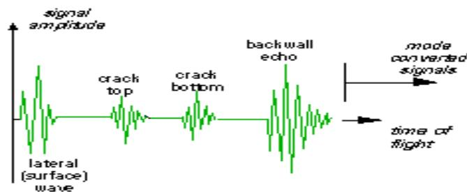
Fig. 4 - schematic of TOFD A-scan
