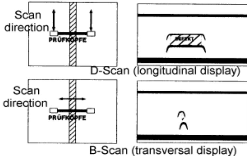
Fig. 6 Scanning of weld in parallel and perpendicular direction to weld axis <sup>[6]</sup>
