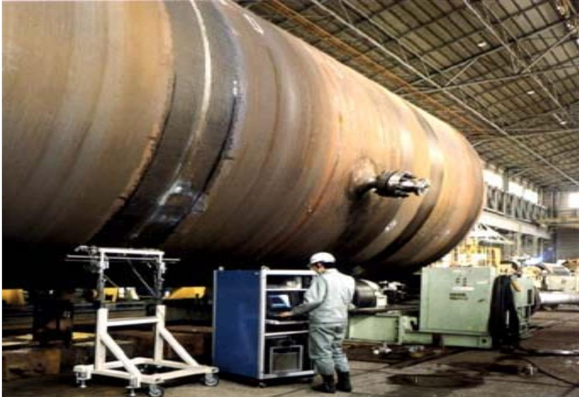
Fig. 8 TOFD being done for a heavy walled pressure vessel at shop [5]
