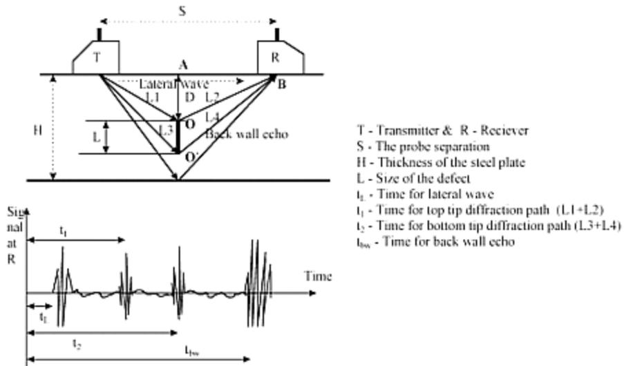
Fig. 7 Mathematical Model of TOFD Technique [13]
