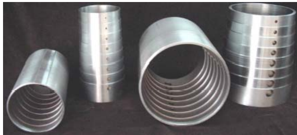
Figure 2: Reference blocks fabricated from 6 and 10 inch pipes
