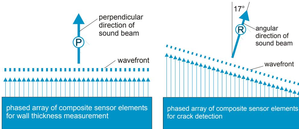
If a set of neighbouring composite sensor elements is triggered with a certain time shift from element to element, an angular sound pulse is generated. The direction of this sound pulse depends on how the time shift increments.
