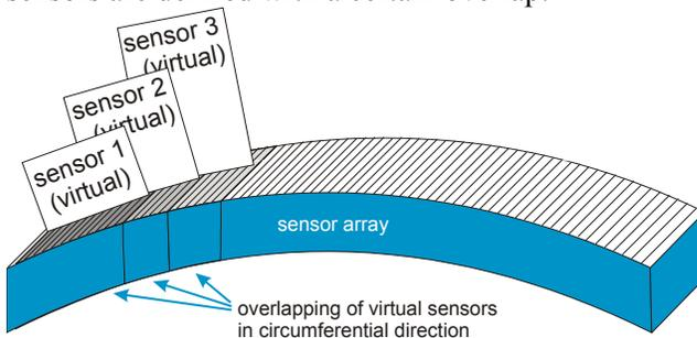
With the sensor overlap, an optimum circumferential coverage of the pipe wall is achieved.
