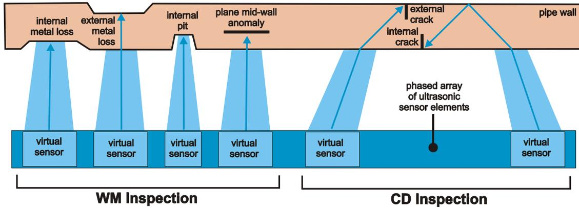
Phased Arrays of composite sensor elements allow to built-up virtual sensors of different sizes and shooting in different directions. Metal losses and laminations are detected with perpendicular sound beams, cracks with angular sound beams.
