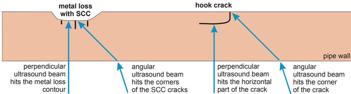
Defects like "metal loss with SCC" or "hook cracks" are detected with optimum POD and POI if both perpendicular and angular ultrasound beams are used.
