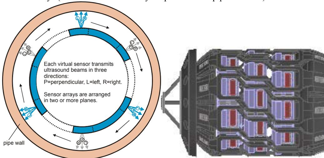
The Phased Arrays on the sensor carrier sections are arranged in a way that each array covers a certain section on the circumference including minimum overlaps with the neighbouring arrays.
