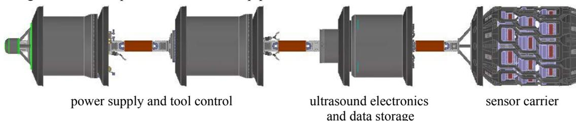
The Phased Arrays are approx. 100 mm long and comprise about 200 composite sensor elements.
