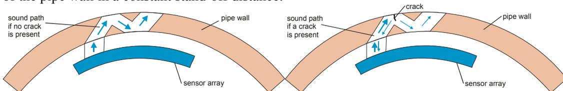
A virtual sensor is activated by the ultrasound electronics to shoot in the desired direction.
