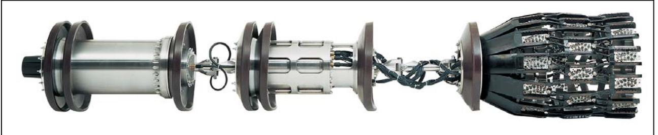
**Figure 1 High Resolution Ultrasonic In-Line Inspection Tool for 24" pipelines. The tool is made up of two pressure vessels housing batteries, electronics, recording devices and a trailing sensor carrier housing the ultrasonic transducers.**
