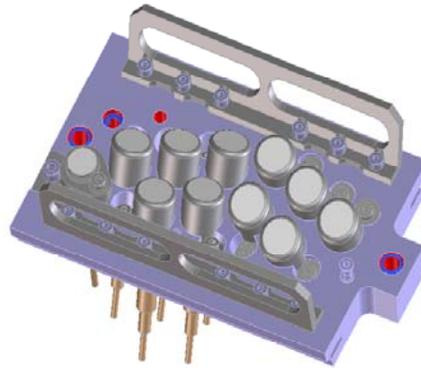
**Figure 2 The assembly for the crack detection sensors**
