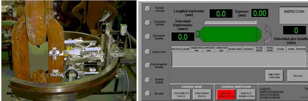
Figure 5. System in operation upon a link (left) and sample of inspection results (right)
