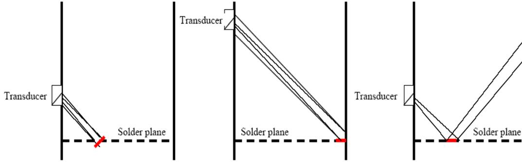
Figure 1. Flaw detection by single angle-beam transducer inspection. Inner imperfections normal to the probe beam (left) or edge imperfections parallel to the solder plane (centre) are detected, but inner imperfections parallel to the solder plane (right) are lost
