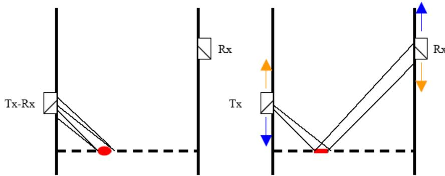
Figure 2. Proposed dual transducer inspection
