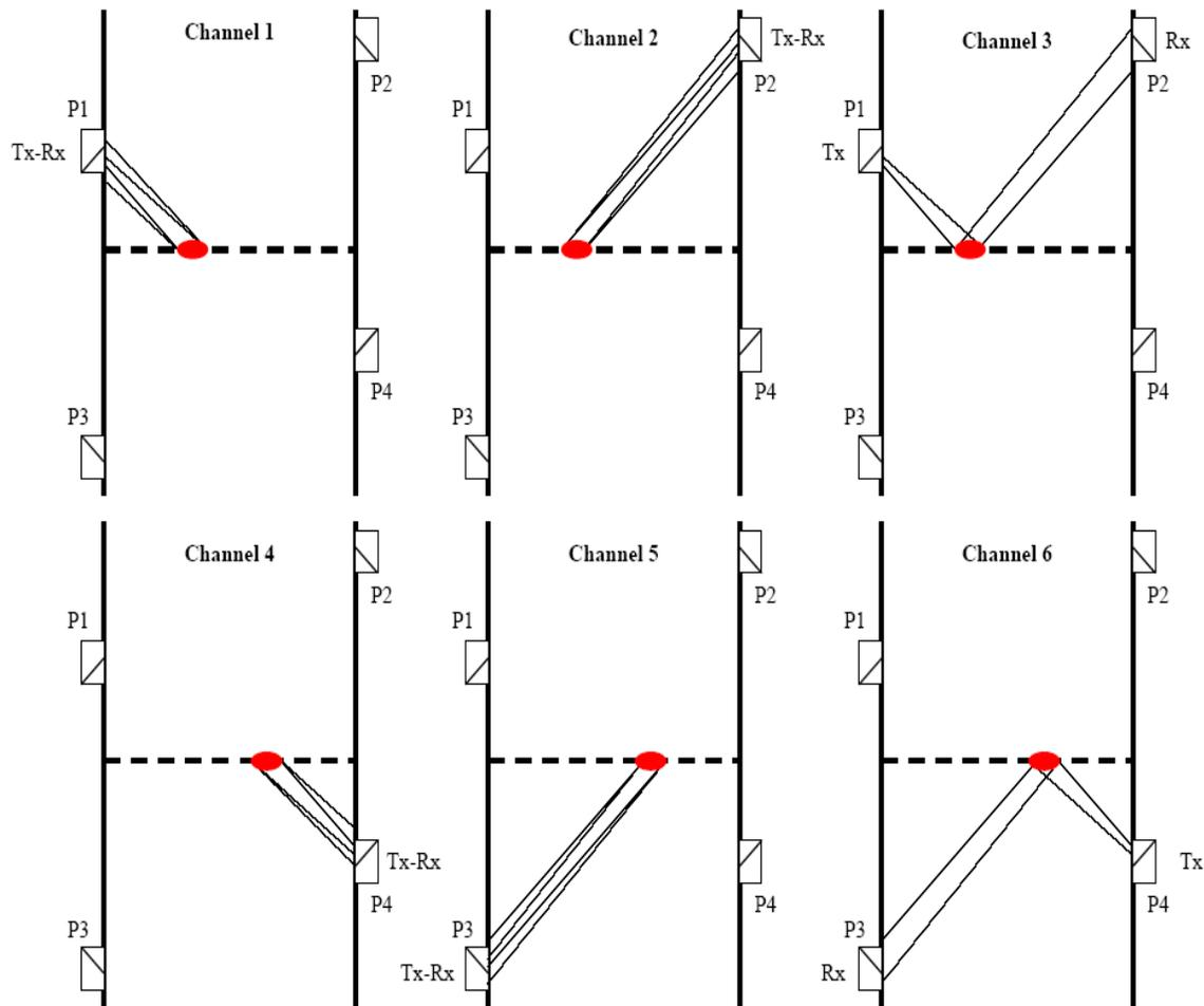
*Figure 4. Six effective inspection channels are obtained with proposed four-probe set-up*
