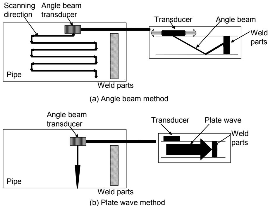
**Fig.1 Fundamental concept of an ultrasonic nondestructive inspection robot**
