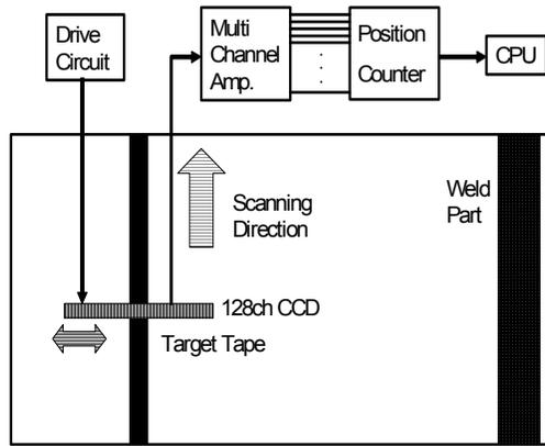
(a) Mechanical concept of the inspection robot
