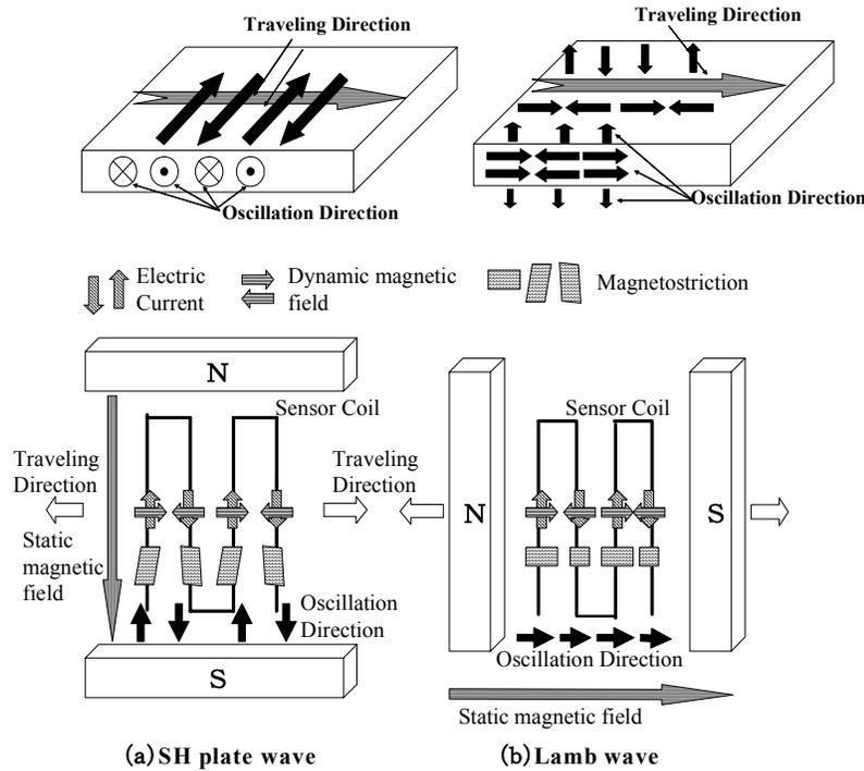
**Fig.2 Drive mechanism by the EMAT**
