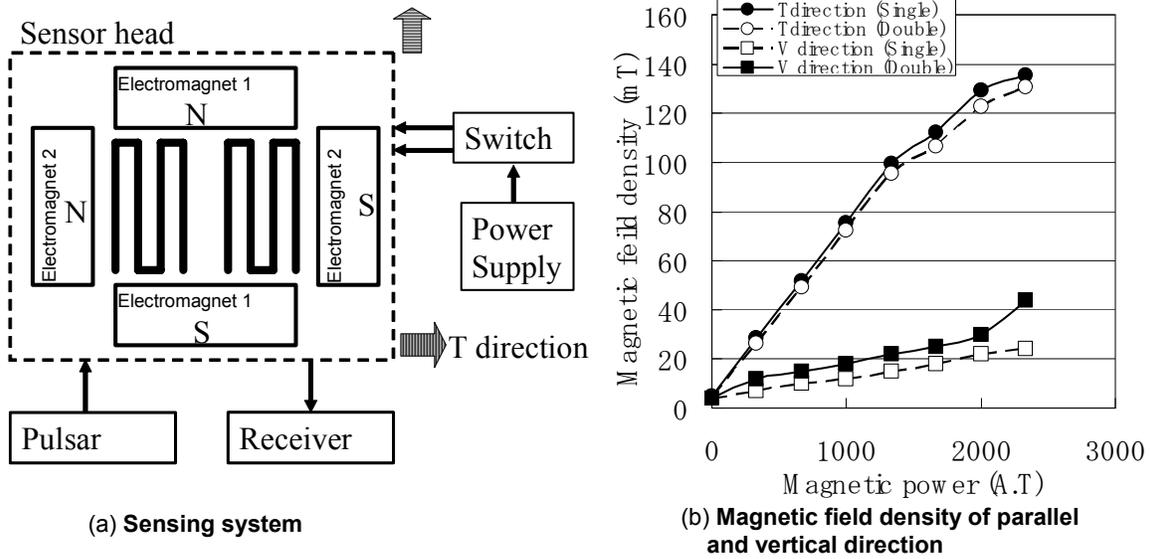
**Fig.3 Basic EMAT driving system and the measured magnetic field between the magnetic poles**
