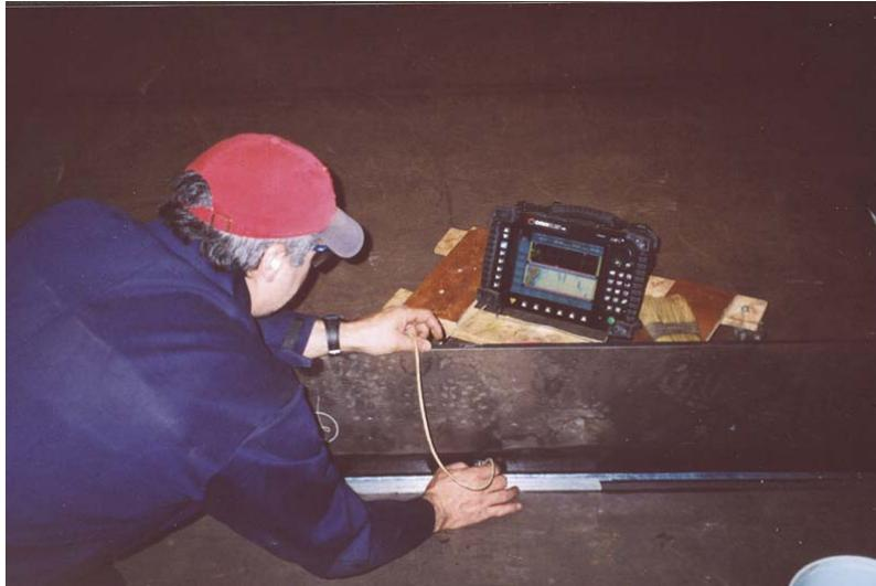
Figure 12: Portable phased array instrument for tie-ins and repairs, performing a linear scan on a weld.
