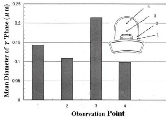
Fig.4 Result of NDI Replica Inspection of Transition Piece ( 20,000h After Service)
