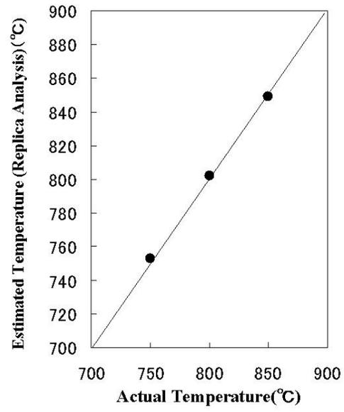
Fig.3 Result of Metal temperature Estimation of Aging Specimen
