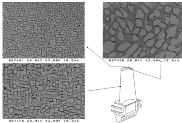
Photo2 Result of NDI Microstructure Analysis of First Stage Bucket
