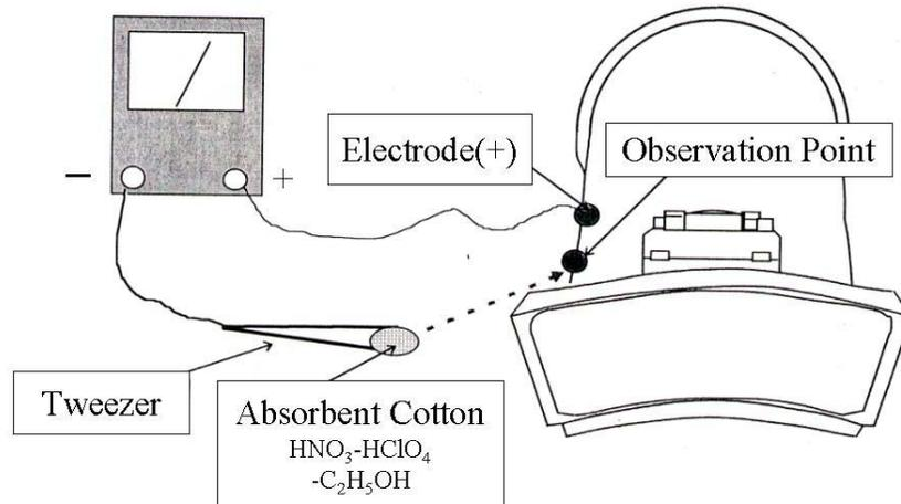
Fig.1 Illustration of The Etching Method in This Work
