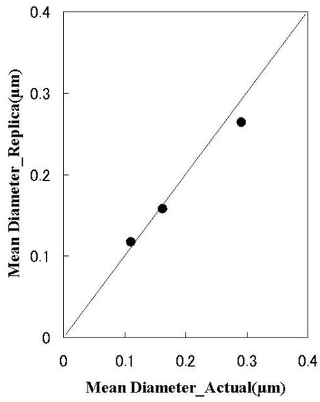
Fig.2 Result of Replica Analysis of Aging Specimens
