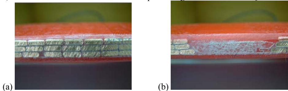
Fig. 3. (a) The cross section of partial high tension coil. (b) The cross section of glass fiber in high tension coil.
