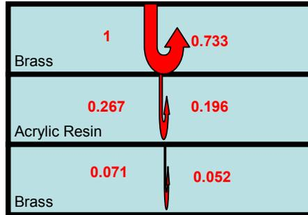
Fig. 4. The transmission and reflection of power wave in brass and acrylic resin.
