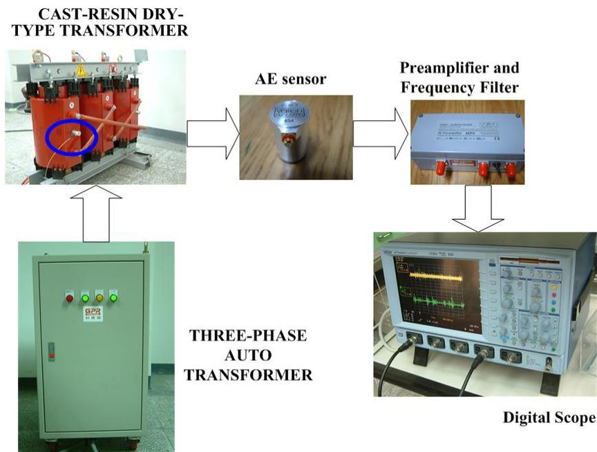
Fig. 5. Schematic diagram of the PD measurement system.
