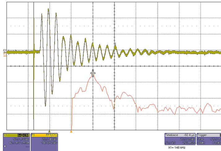
Fig. 8. AE signal and frequency spectrum that measured by using VS150-M.
