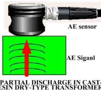
Fig. 2. The sensors – converting the mechanical wave into an electrical AE signal.
