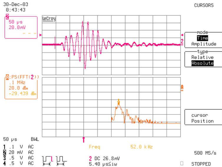
Fig. 10. AE signal and frequency spectrum that measured by using VS30-V.
