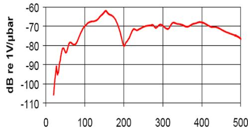
Fig. 1. Frequency spectrum of the VS150-M (kHz) AE probe [3].
