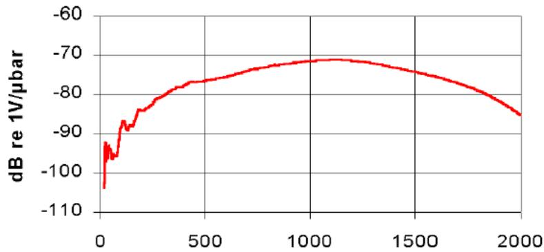
Fig. 6. Fuji 2045S, f(kHz) [3]
