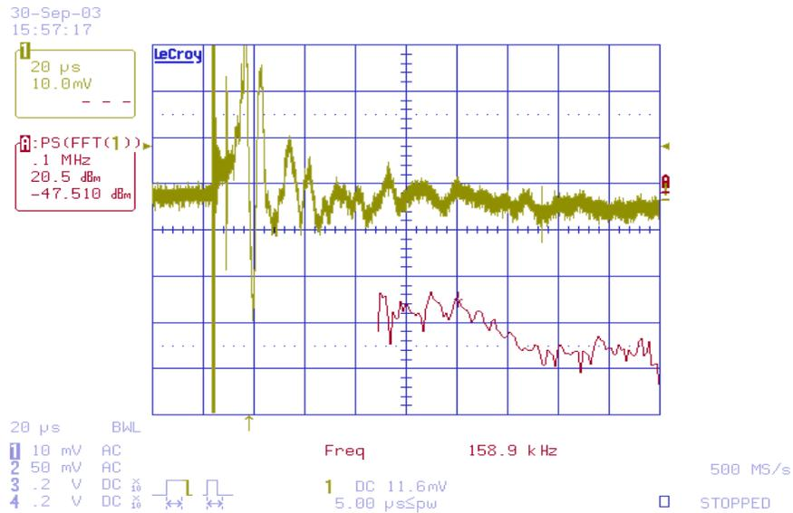
Fig. 9. AE signal and frequency spectrum that measured by using Fuji 2045S.
