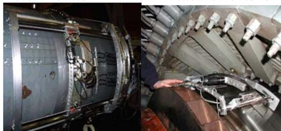
**Fig 2 End ring scanner set-up & Fig 3 Inspection in-situ**
