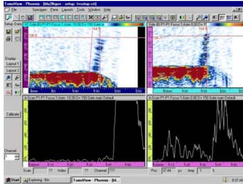
**Fig 14 Phased array image of crack orientation**
