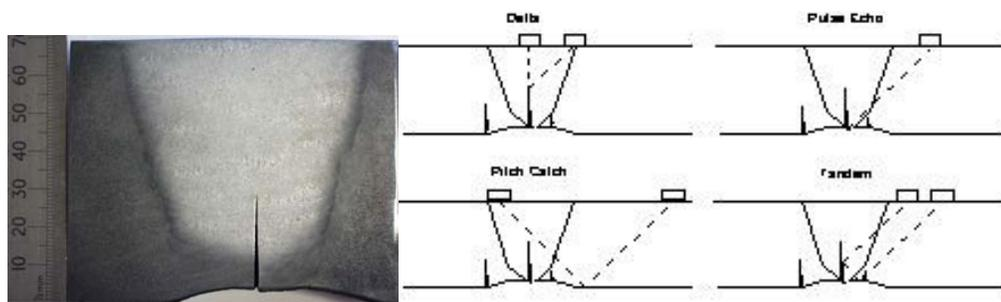
**Fig 15 Severe Pipework Bore Crack & Fig 16 Ultrasonic NDE Techniques**
