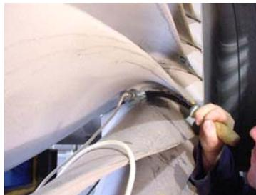
**Fig 12 – manually manipulated phased array technique**
