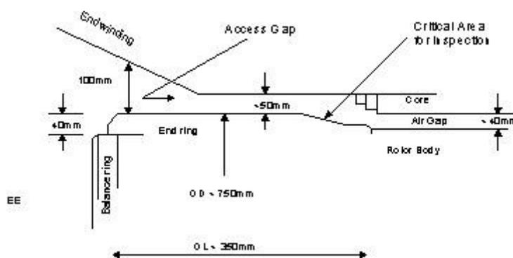
**Fig 1 Rotor – Stator minimum measurements for in-situ**
