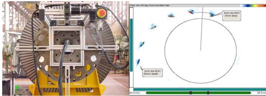
**Fig 4 Rotor Bore Inspection System & Fig 5 – Volumetric Inspection – Polar View**
