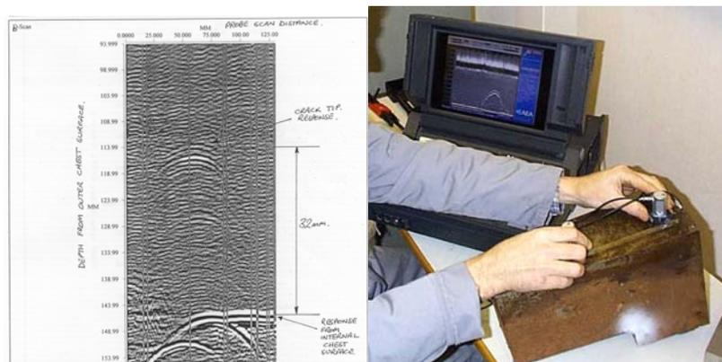
**Fig 13 Typical TOFD result and TOFD in operation**
