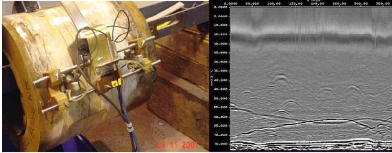
**Fig 17 Innogy Pipe Scanner & Fig 18 TOFD Image - Two Bore Cracks**
