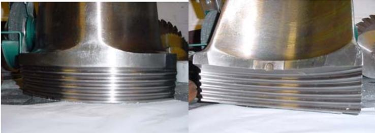
Fig 8 and 9 – Curved blade root geometry
