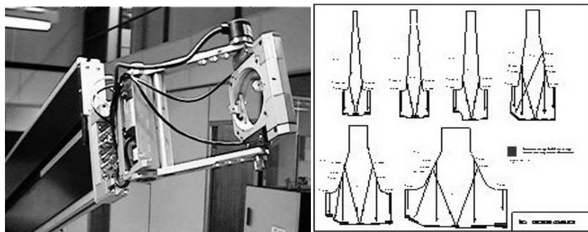
**Fig 6 Inspection Manipulator & Fig 7 Multi angle inspection technique – probe requirements**
