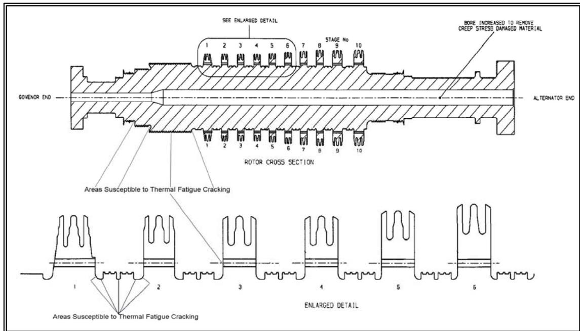
Figure 6 - Thermal Fatigue - Critical Locations
