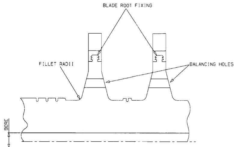
Figure 7 Location of critical areas for accumulation of creep strain
