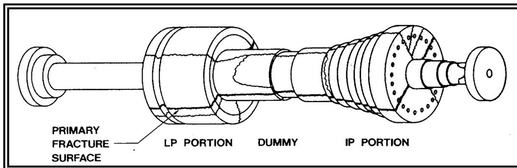
Figure 4 - Gallatin Unit 2 IP/LP Rotor Fragmentation
