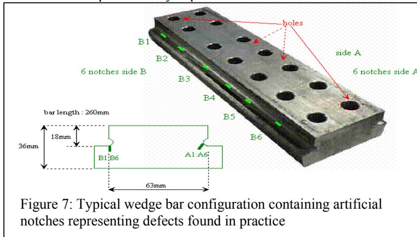
Figure 7: Typical wedge bar configuration containing artificial notches representing defects found in practice
