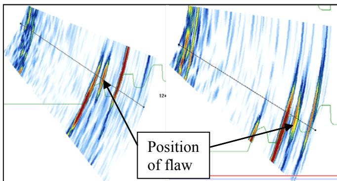
Figure 11: Phased array images showing flaws situated in top two serrations and CAD overlay (in green)
