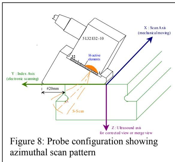
Figure 8: Probe configuration showing azimuthal scan pattern
