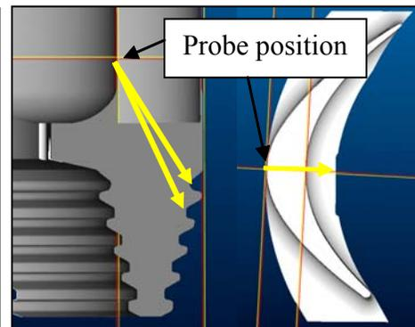
Figure 12: CAD image showing position of probes to produce images in figure 11
