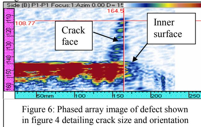
Figure 6: Phased array image of defect shown in figure 4 detailing crack size and orientation
