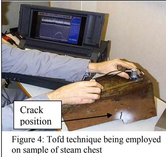
Figure 4: Tofd technique being employed on sample of steam chest
