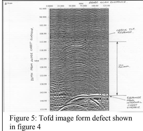
Figure 5: Tofd image form defect shown in figure 4
