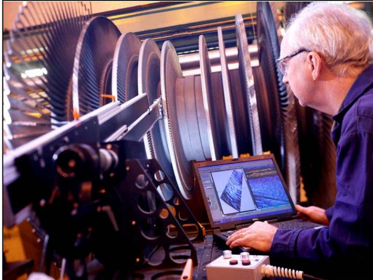
**Figure 1: Rotor disc head manipulator**
