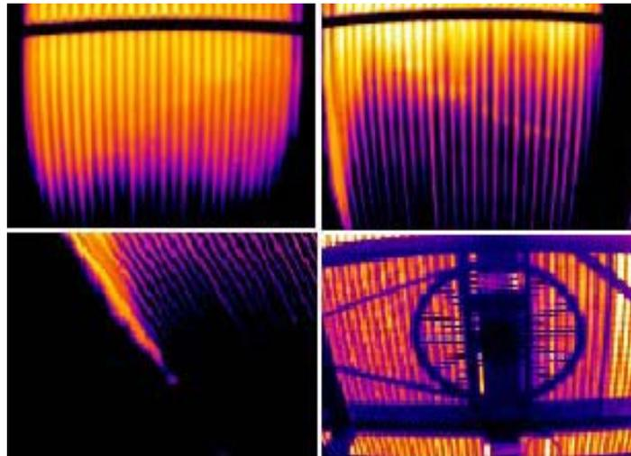
**Fig. 4 – Thermographic Condition Monitoring of COGEN plant**
