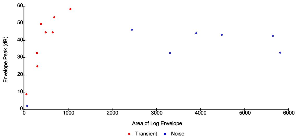
**Fig. 10 – Separation of Acoustic Events**
