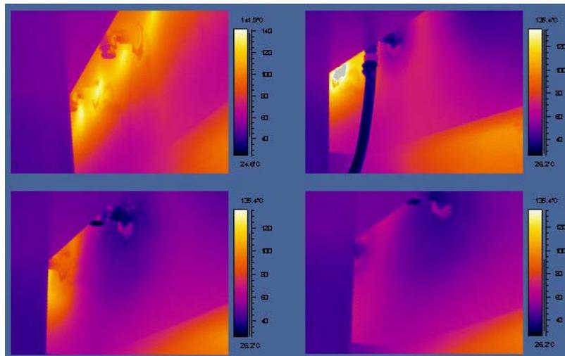
**Fig. 5 – Thermographic Condition Monitoring of an HRSG**
