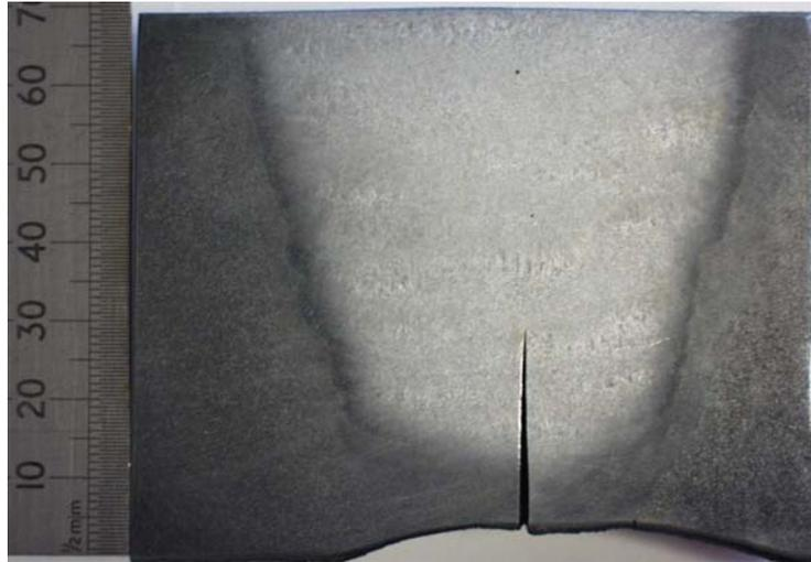
**Fig. 9 – Steam Pipework Thermal Fatigue Crack**
