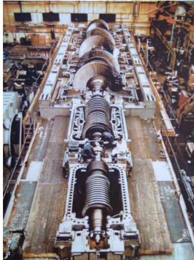
**Figure 2. Steam Turbine Rotor ‘train’**
