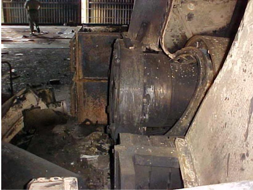
**Figure 5. Broken LP Coupling**
