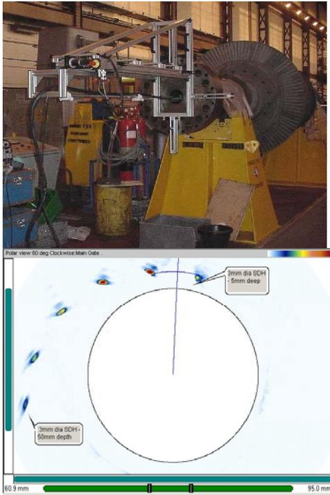
**Figure 6. Bore scanning rig of test sample**
