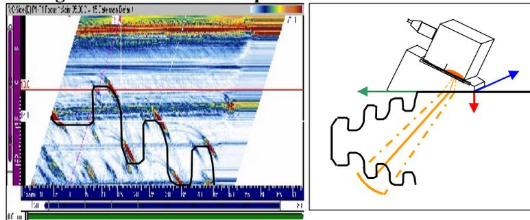
**Figure 9. Electronic 'Raster' Display of 'Fir-Tree' Root Fixing and Phased array probe,**
