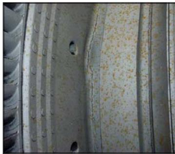
**Figure 3. Photo showing T.F. cracking in disc radii and balance hole.**
