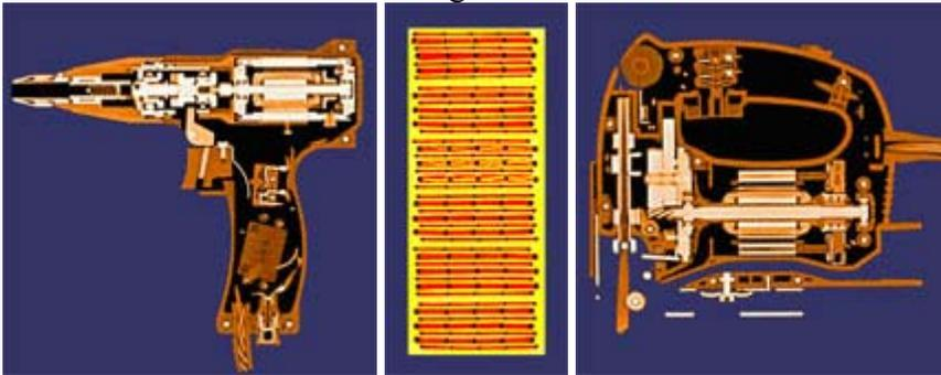
Fig. 5. Tomograms of a power drill, accumulator and electric fletsaw.
