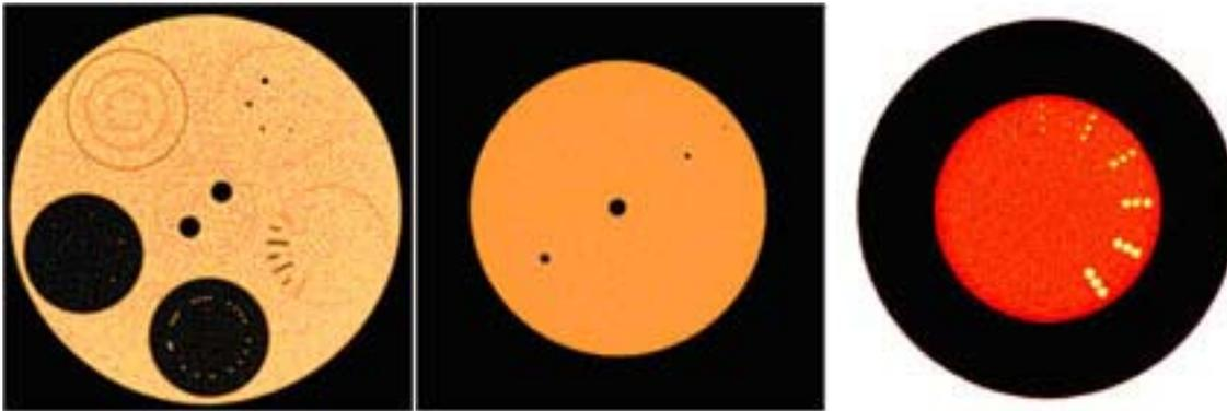
Fig. 2. Tomograms of standard specimen CO-1-A of a steel cylinder of 150 mm diameter with holes  $\varnothing$  8, 4, 2 and 1 mm, and a hollow steel cylinder of 150 mm external diameter and 30 mm wall thickness, filled with dielectrics with a group of holes  $\varnothing$  3.5...1.0 mm.
