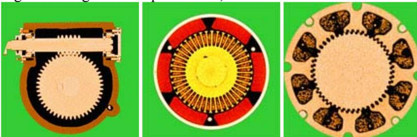
Fig. 6. Tomograms of a worm-and-wheel gearbox, direct-current motor and step motor.
