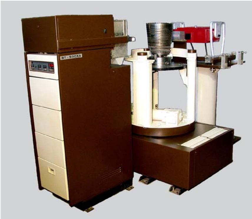
Fig. 1. Tomograph BT-500XA and betatron MIB-5.
