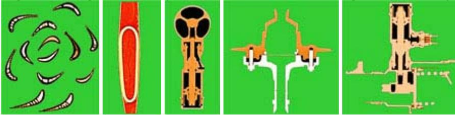
Fig. 4. Group tomogram of 13 cooled turbine blades, tomograms of a helicopter blade and rocket valves. Tomograms of real products of electrical engineering and machine building obtained with the use of betatron MIB-5 are shown in Figs. 5-6.
