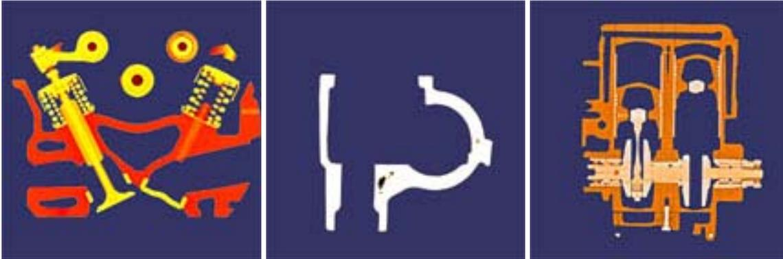
Fig. 3. Tomograms of a cylinder block head, a steering tube of a lorry and an internal-combustion engine.
