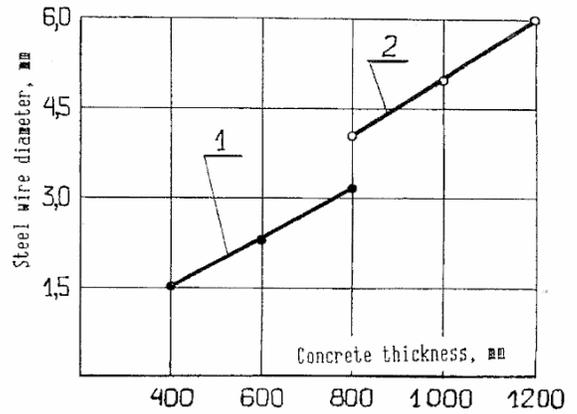
Fig.5. Dependence of steel wire sensitivity coating thickness.
