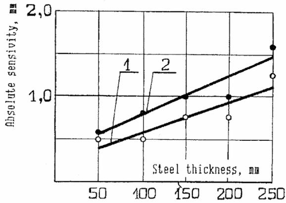
Fig.4. Dependence of defect sensitivity on steel on thickness.
