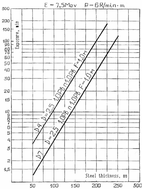
Fig. 2. Exposure thickness curve for steel.
