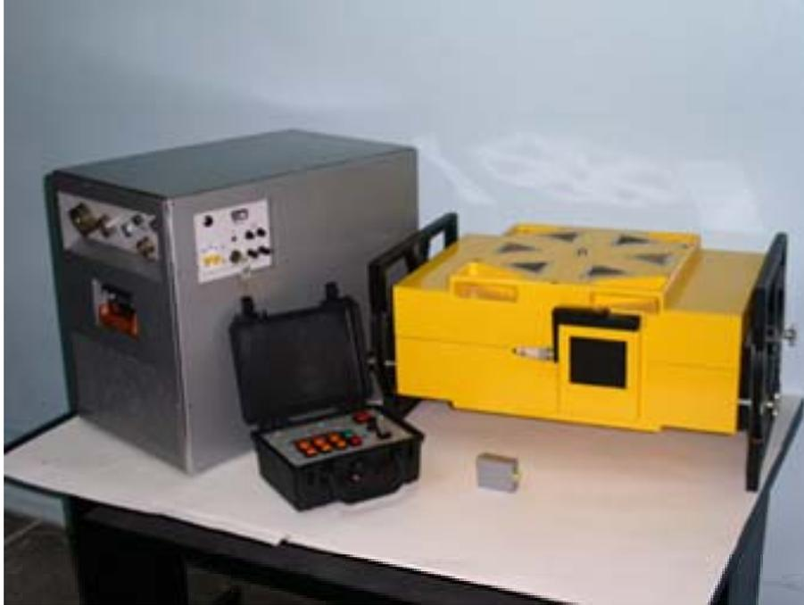
Fig. 1. Portable X-ray betatron PXB-7.5
