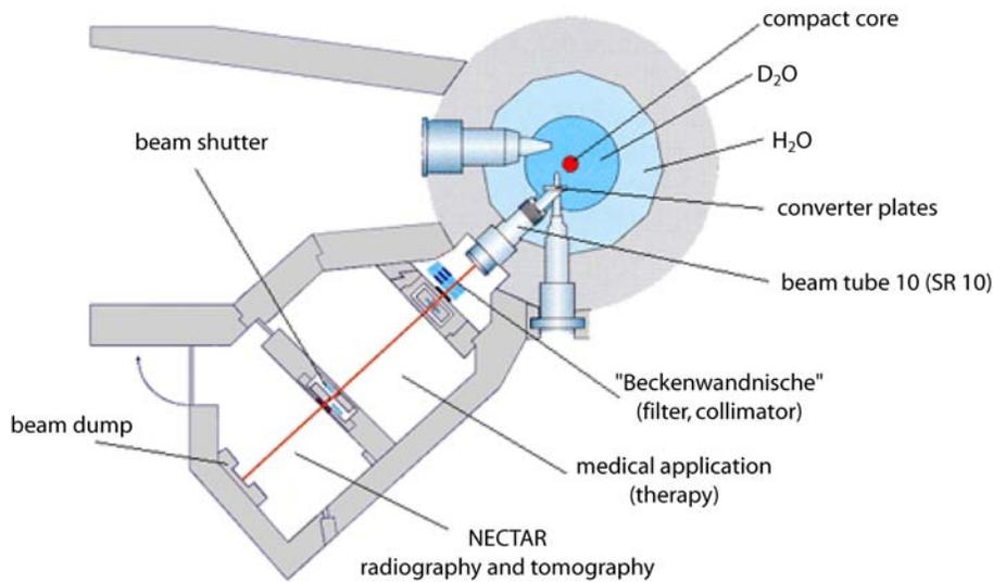
Figure 4: Schematic layout of the NECTAR facility.
