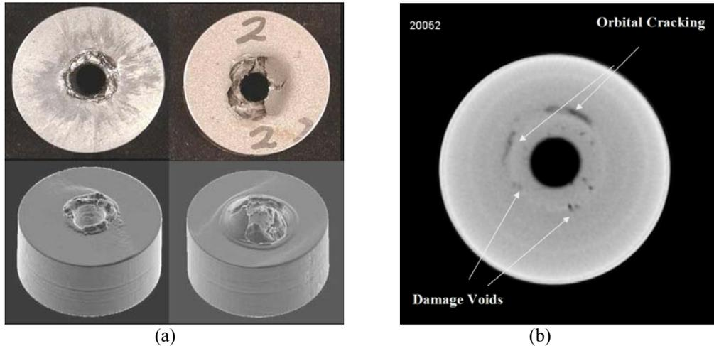
Figure 1. (a) Macro-photographs of the 50 mm diameter AP<2 sample #2 (top) and the respective 3D XCT virtual object reconstructions (bottom) of both the impact (left) and (exit) surfaces, (b) Individual XCT axial scan #52 of Ti-6Al-4V APM2 sample #2 showing small damage voids and large curved orbital cracking segments. Axial slice is  $\sim 4$  mm from the sample exit face.
