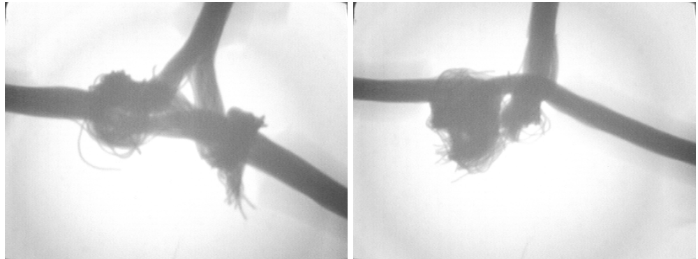
Fig. 7. Detection of wire connection rupture in all-in-one contact assembly (the images are obtained in case of projecting amplification)
