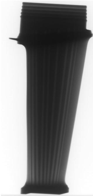
Fig.1 Inspection image of turbine blade
