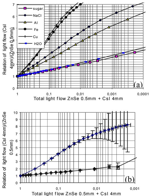
Fig. 7. The Determination of the composition of substance by 2-energy method. Two scintillators - ZnSe (0,5mm) and CsI (4mm).
