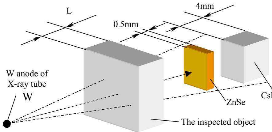
Fig. 5. A model of the two-energy detector array and spectrum of the X-ray tube with a tungsten anode. Calculations were carried out for the following substances: Al, Cu, Fe, NaCl, H<sub>2</sub>O, C<sub>12</sub>H<sub>22</sub>O<sub>11</sub> (sugar).
