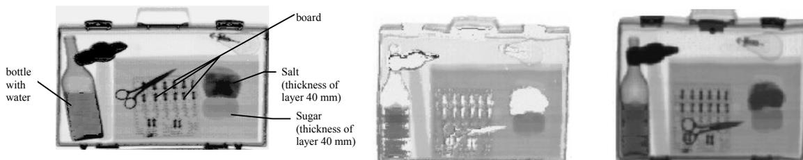
response, radiation stability, rather low effective atomic number together with sufficiently high density – makes this material the best among known scintillators for the low-energy detector. Combination of crystals ZnSe(Te)/CsI(Tl) in the two-energy detector array has substantially improved the sensitivity of equipment designed for detection of organic inclusions (Fig.4).
