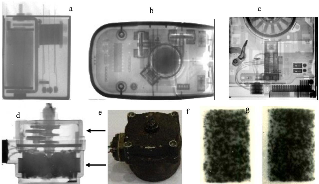
Fig 2 Some neutron radiographs got in SPRR-300. a: relay, b: a mouse, c: a floppy disk, d and e: a motor and its practicality image, f and g: UO<sub>2</sub> fuel pieces (a black dot is a Gd<sub>2</sub>O<sub>3</sub> grain):
