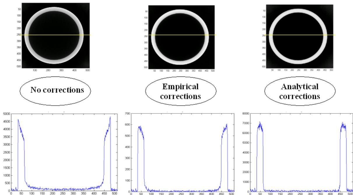
Figure 5. Test Case #1: Mid-plane CT images and corresponding opacity profiles, from VCT data set, for 120kVp imaging of 150mm diameter, 9mm wall Al annulus; comparison of cases for no corrections, empirical corrections, and analytic corrections
