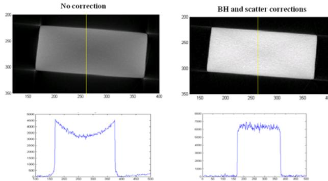
Test Case #3 involved the Al annulus, where the VCT scanning was repeated with no source collimation. The image improvement first with the BH correction alone (middle image and profile) and then with both BH and scatter (right image and profile) are shown in Figure 7. The quality of the final result is encouraging.
