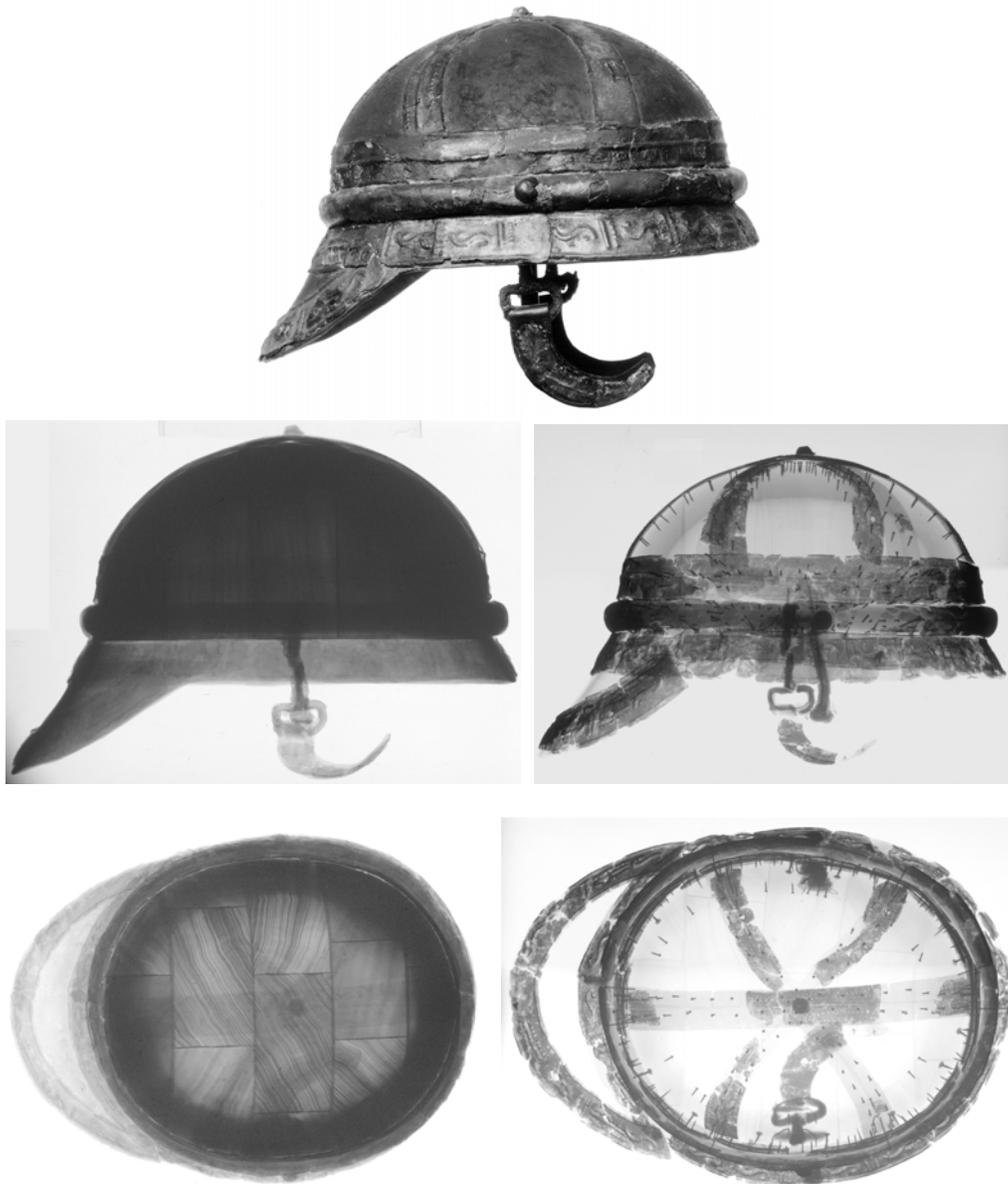
**Fig. 5:** Results of the transmission of a helmet claimed to be of Roman origin with neutrons (left column) and X-ray. Whereas the metal parts are perfectly shown in the X-ray images, the neutrons are able to visualize the structure of the used wooden material and leather.
