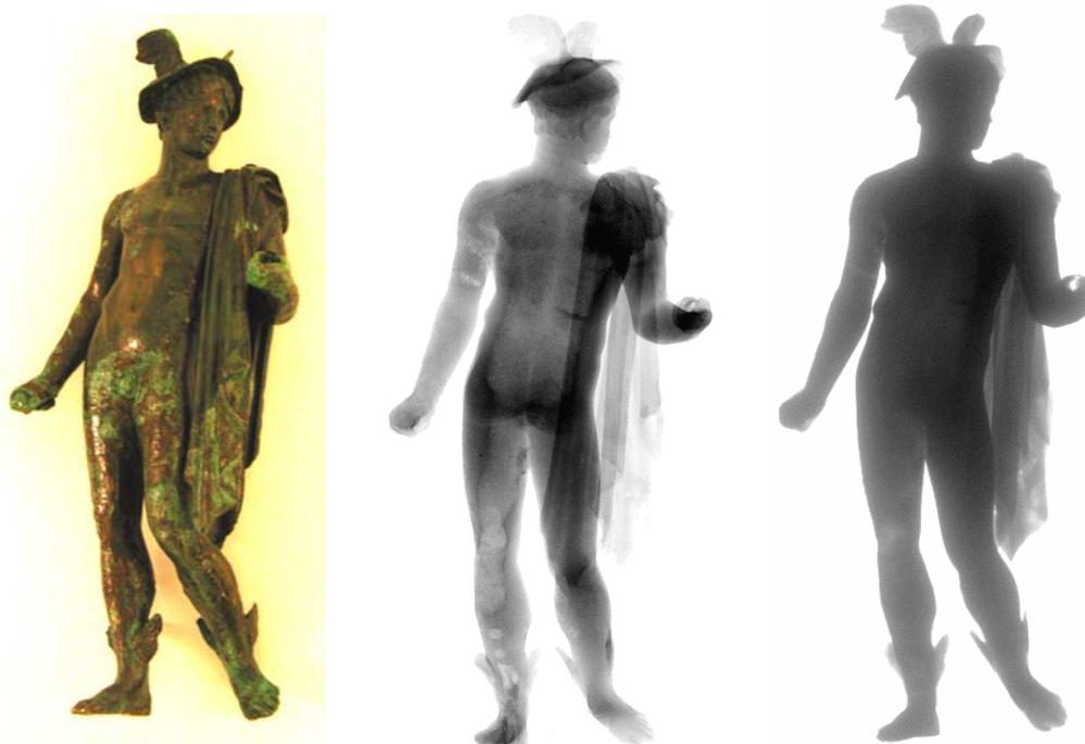
**Fig. 4:** The bronze sculpture “Mercur from Thalwil” (Photo left) was investigated with thermal neutrons (middle) and X-ray at 150 kV (right). The much higher penetrability by neutrons enables to see inner structures, which is impossible for this applied X-ray energy. This object is about 25 cm high.
