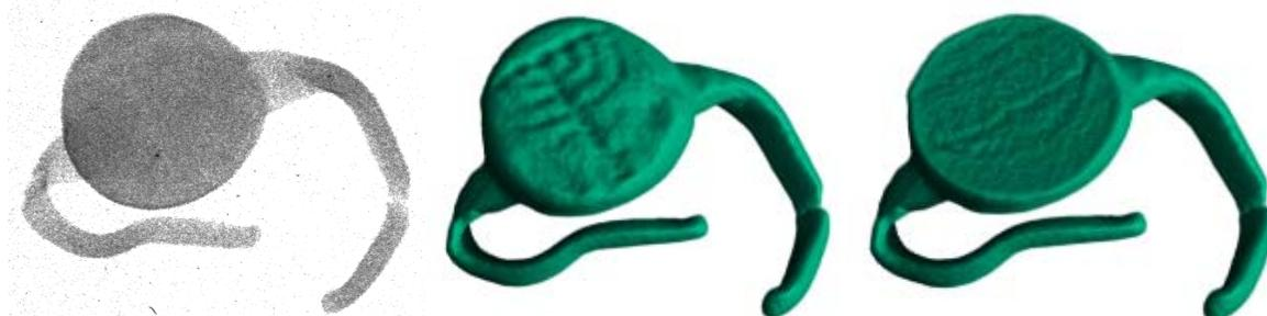
**Fig. 1:** Results of neutron investigations of a Jewish finger ring from the Roman era: left: neutron transmission, middle and right: neutron tomography. The right picture shows a virtual slice made by software tools through the object on the level where the both parts are fitted.
