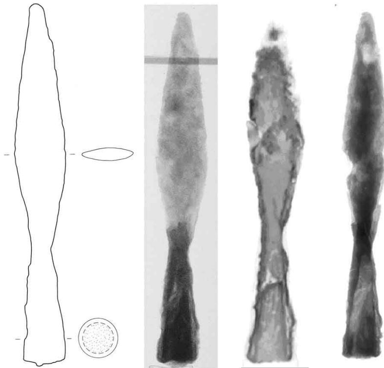
**Fig. 3:** Results of the investigation of a Roman spearhead (found near Giubiasco (CH)): from left to right– drawings, neutron transmission image, neutron tomography slice through the central plane, X-ray transmission image.
