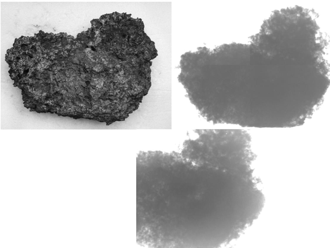
**Fig. 2:** The „Zurich lump“ (photo on the upper left) with a weight of about 70 kg, identified as an assembly of molten coins of “poitin” metal from the Celtic era was investigated by standard neutron transmission analysis (right) and later with a special method extending the dynamic range of the imaging method. In this way, an insight into this about 40 cm thick sample becomes possible (see the image below).
