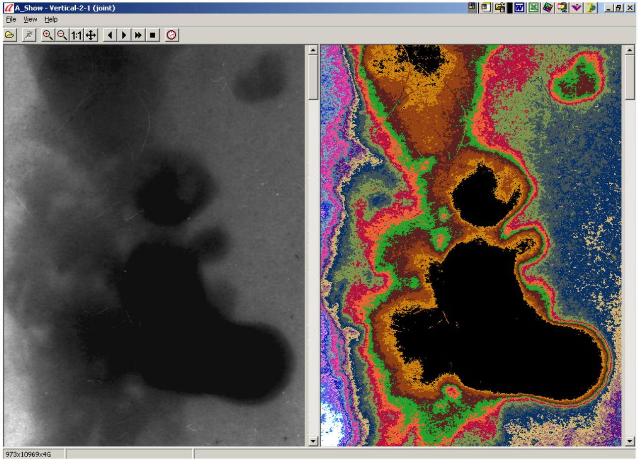
Fig. 2 Welded seam with crack before processing (left) and after processing (right).
