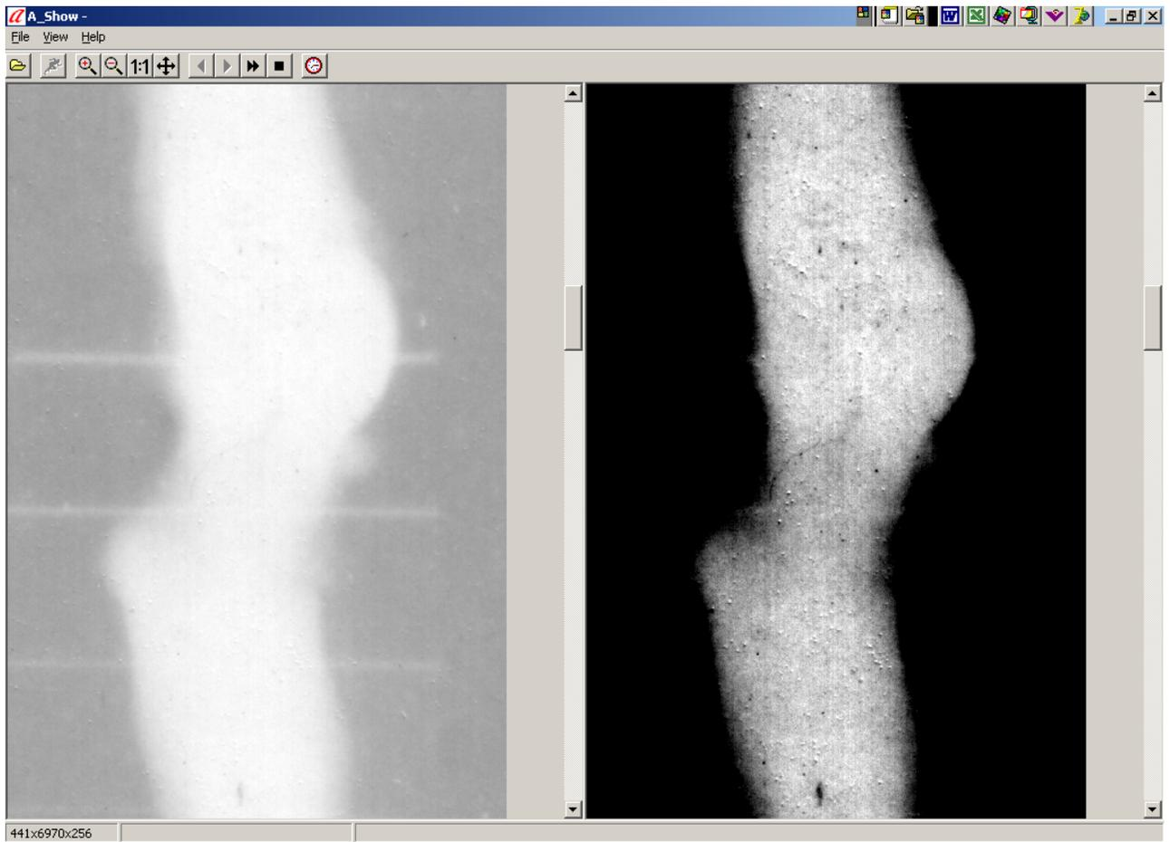
Fig. 1 Welded seam with crack before processing (left) and after processing (right).
