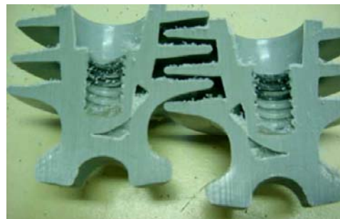
Insulator after cutting
