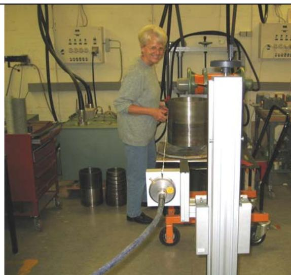
**Fig. 5:** Alignment of the radiation source (Co 60) for the tangential projection technique. Behind the 12 inch pipe is the film cassette. The pipe sits on a turn table for easy positioning of the different holes in relation to the film.
