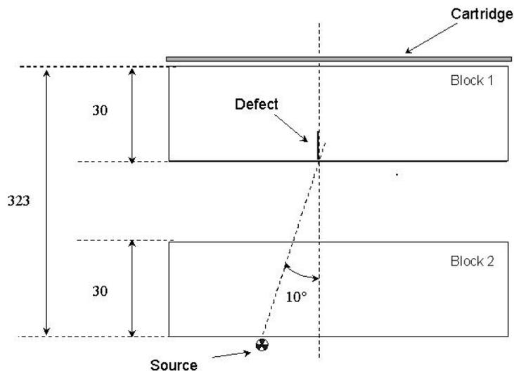
Figure 5 : Tested configuration with a  $10^\circ$  shift around the perfect source and defect plane alignment
