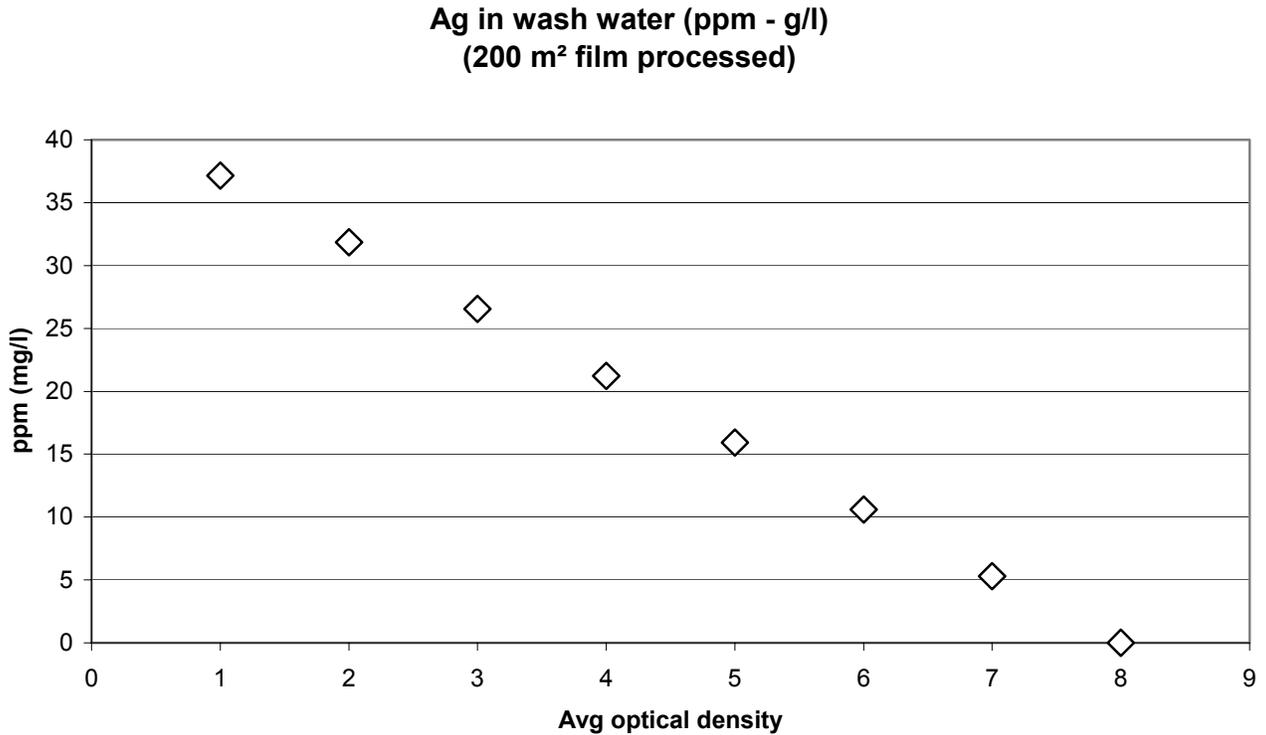
**Figure 1: Relation between Average optical density and silver Ag<sup>+</sup> concentration in wash water**
