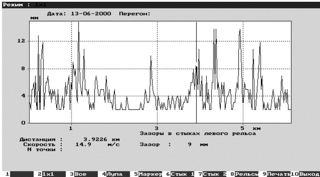
**Fig. 6. Presentation of measured track parameters in the graphic mode: rail butt clearance.** The following parameters are displayed: Operating mode; Date; Run; Clearance in butts of left rail; Distance: km; Traveling speed: m/sec; Clearance: mm; Point #
