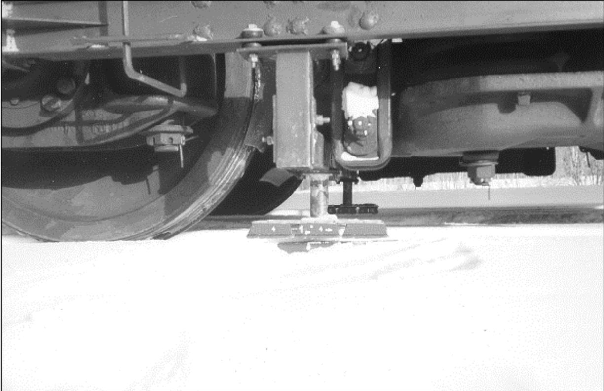
**Fig. 1. Scheme of the ECT modules placement over the rail surface (winter time)**
