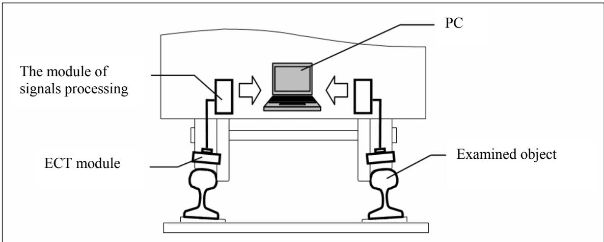
**Fig. 2. The scheme of measuring system placement on the vehicle for the track measurement**
