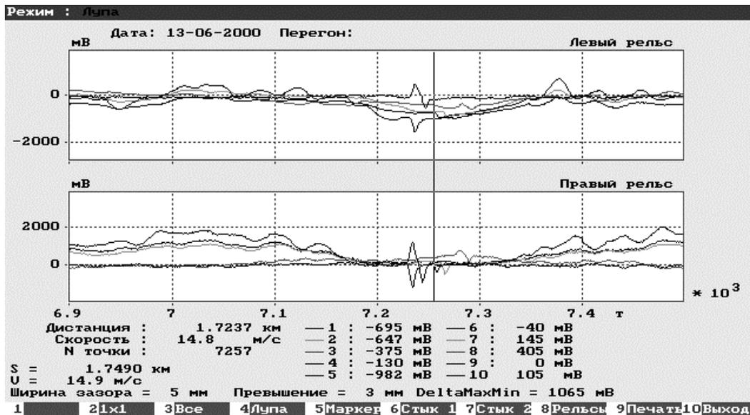
**Fig. 7. The mode of ECT signal recording in the adjustment mode.** The following parameters are displayed: Operating mode; Date; Run; For left rail and right rail; Distance: km; Traveling speed: m/sec; Clearance: mm; Point #; Clearance width = mm; Height exceed = mm.
