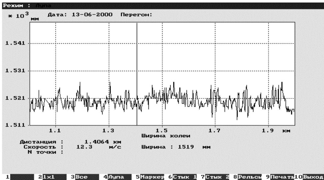
Fig. 5. Presentation of measured track parameters in the graphic mode: track width. The following parameters are displayed: Operating mode; Date; Run; Track width; Distance: km; Traveling speed: m/sec; Width: mm; Point #
