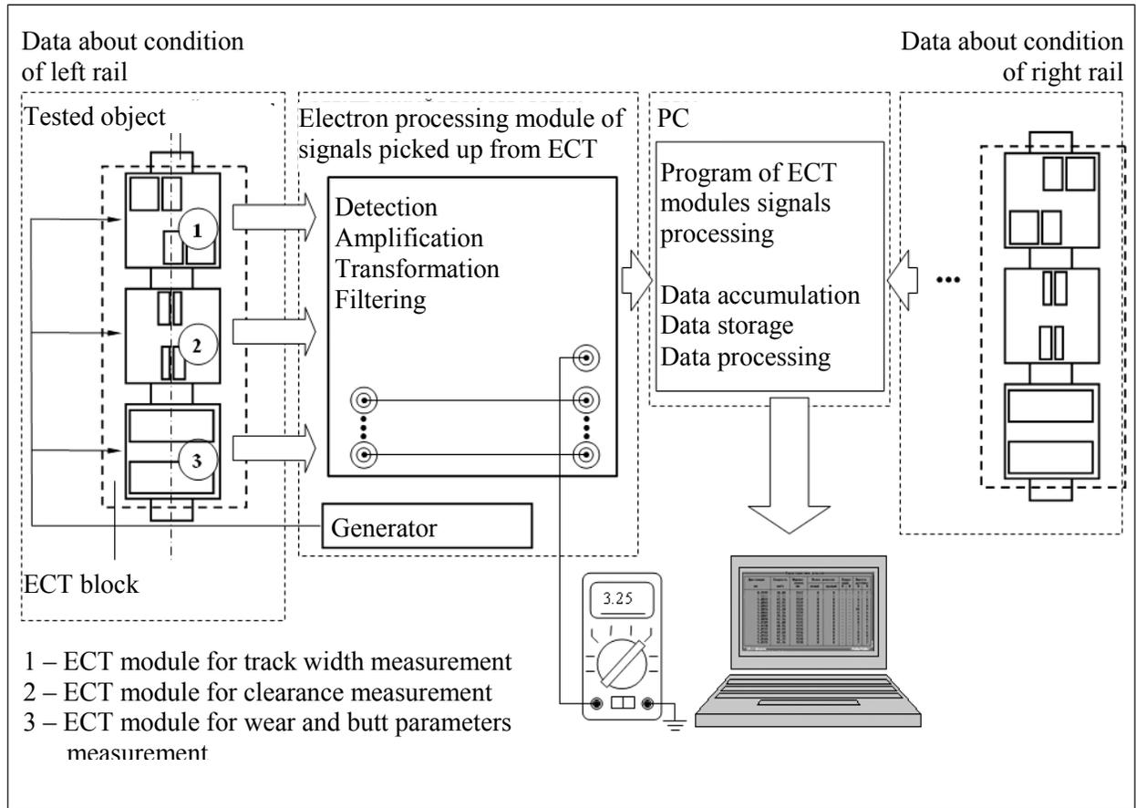
**Fig. 3. General scheme of PKRN-01 system**
