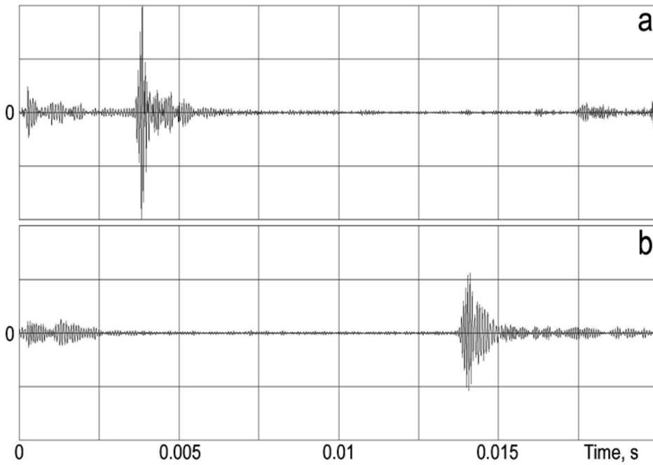
**Figure 2. Echo-signals from the rail's butt-end at the distances between the array and the butt-end of 5 m (a) and 20 m (b)**
