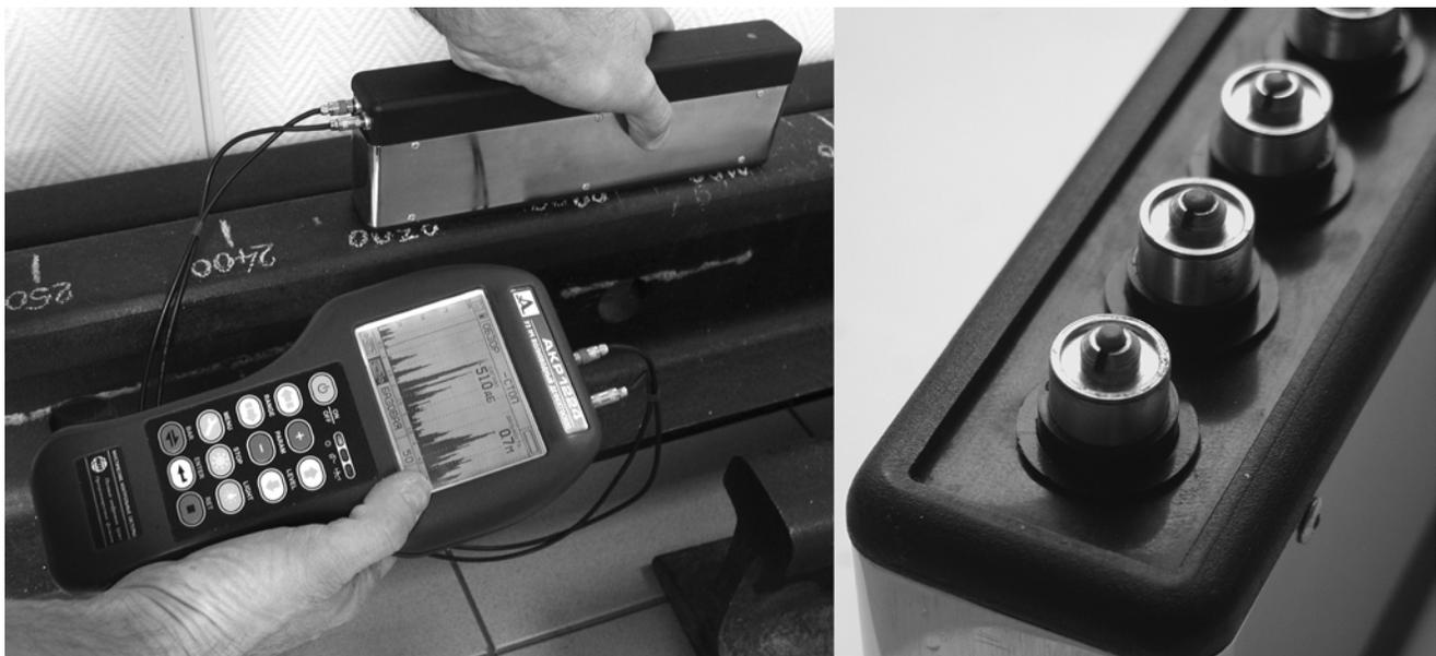
**Figure 5. Rail testing. Antenna array**
