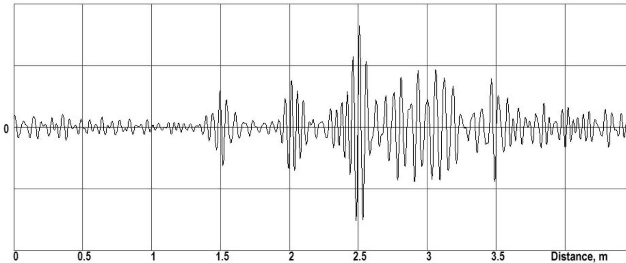
**Figure 4. Echo-signals from the model of defects in rail's head**
