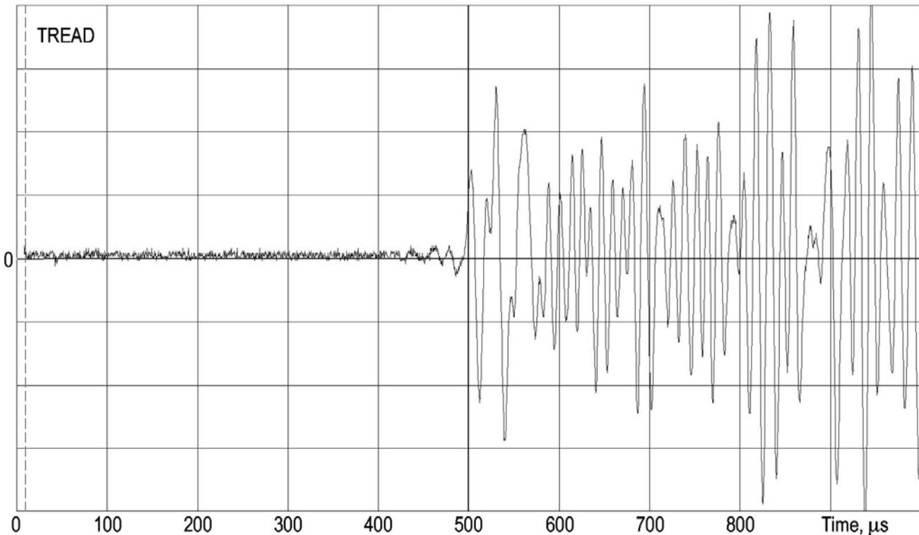
**Figure 1. Signal oscillogram, received at sounding of rail along the driving surface at the base of 1500 mm**
