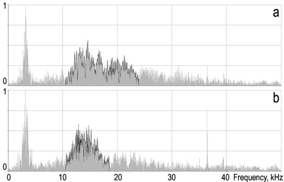
**Figure 3. Spectrum density modules of signal summarizing realizations in rail at the distances between the array and the butt-end of 5 m (a) and 20 m (b)**
