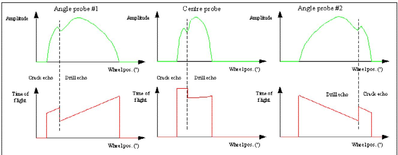
Figure 7. Expected A-Scans for damaged drills with radial (angle probes) or transverse cracks (centre probe)
