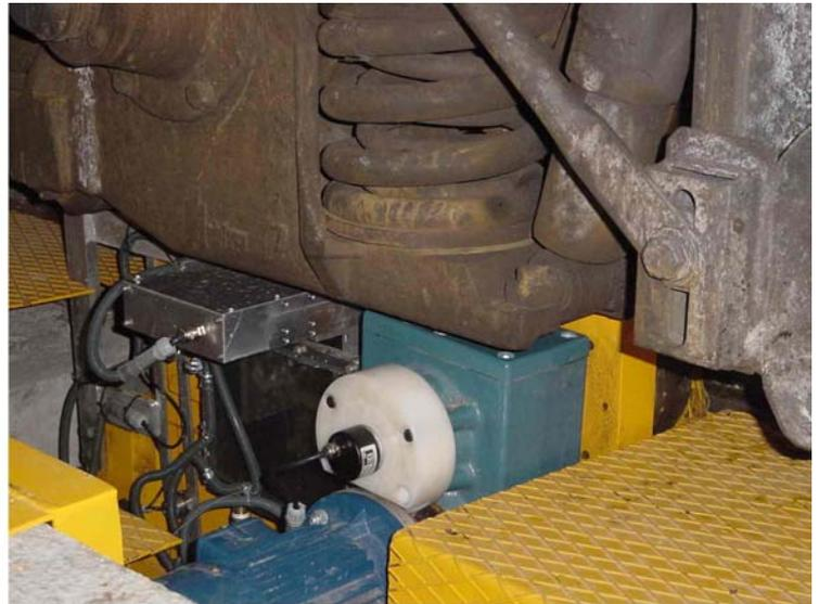
**Figure 11. Train in position on the inspection system (left) and detail of mounted wheel being inspected (right).**
