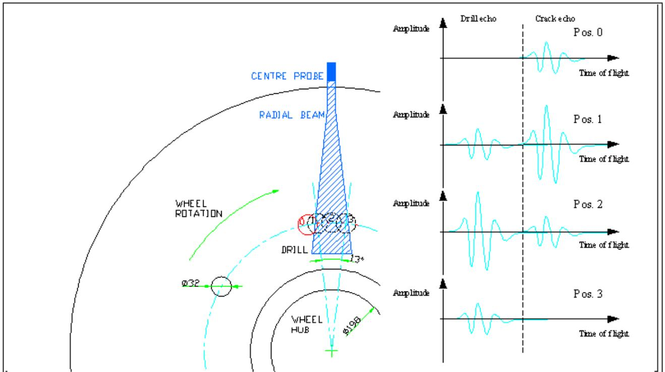
Figure 6. Expected echoes for damaged drill as seen from centre probe
