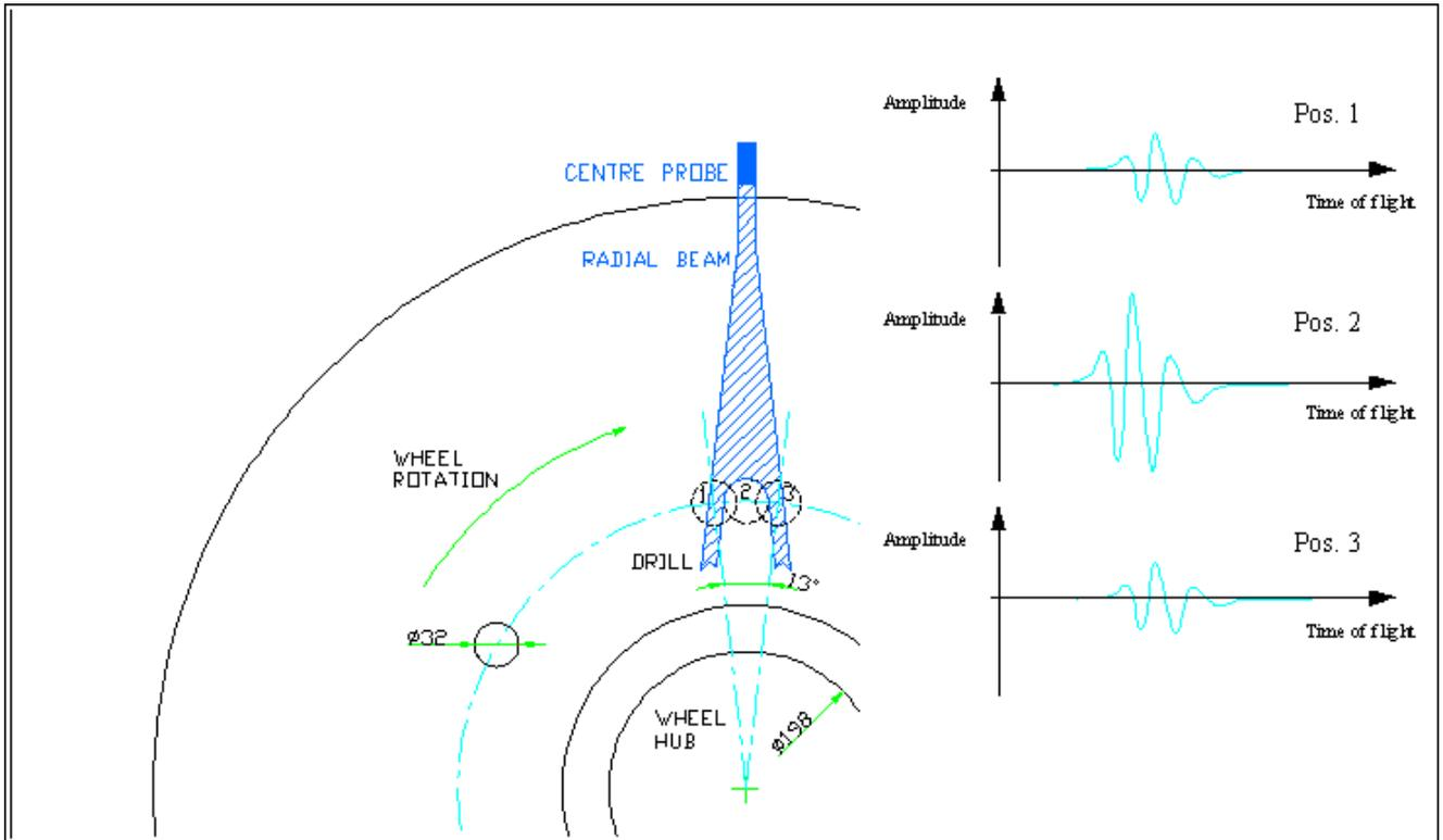
Figure 3. Expected echoes for different positions of sound drill as seen from centre probe
