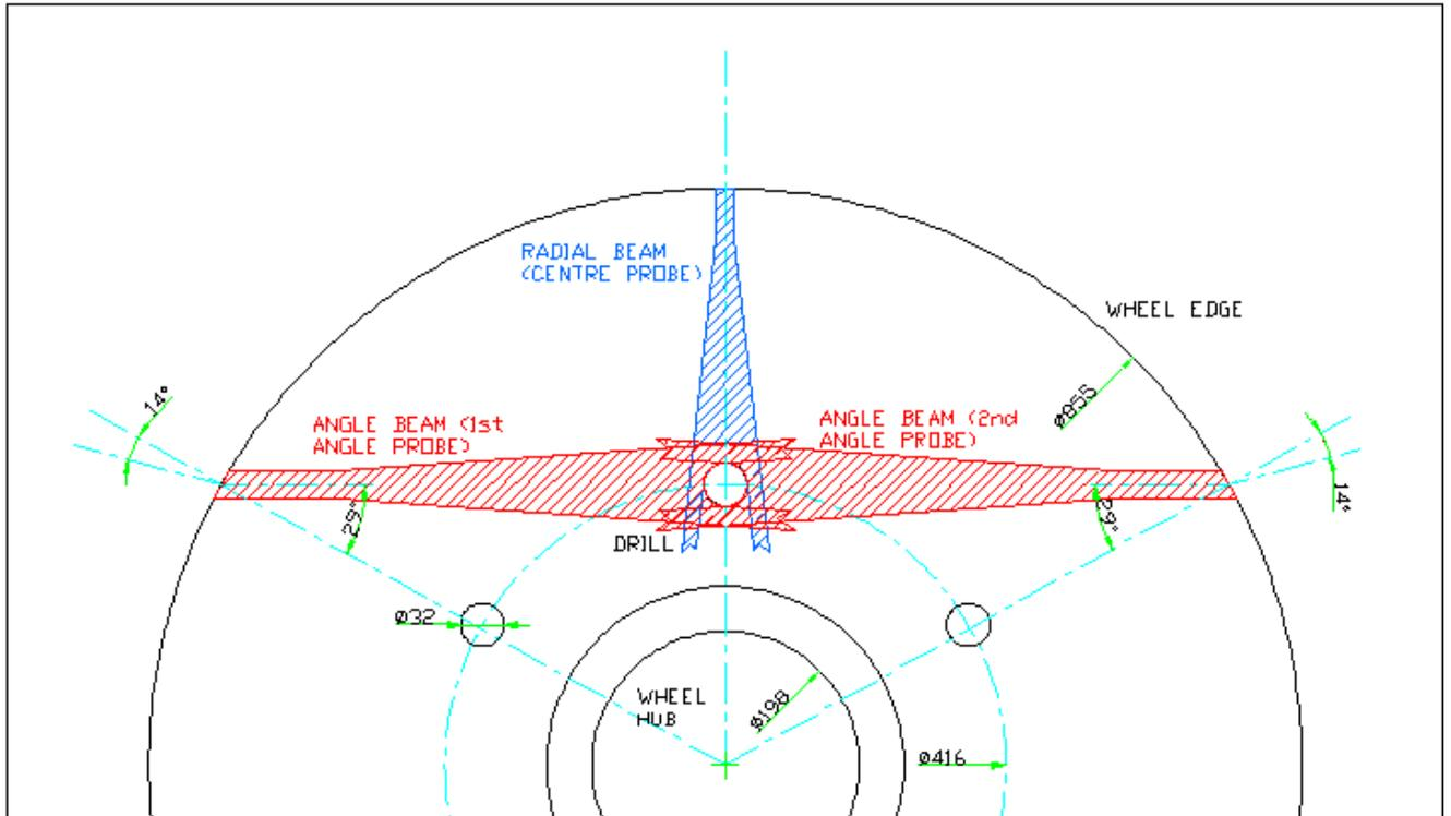
*Figure 1. Drill area coverage with single probe vs. three probe inspection*
