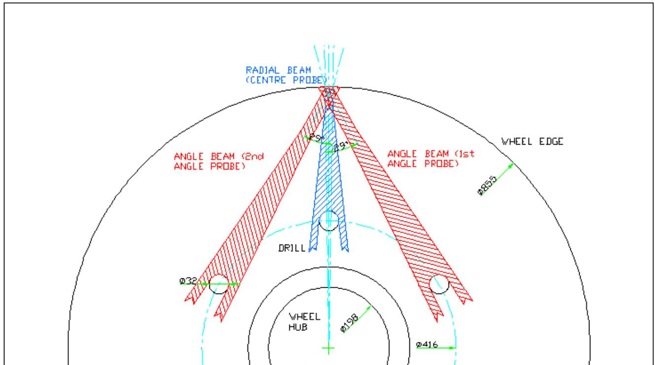
Figure 2. Three-probe set-up for full coverage of the drill area and minimum size
