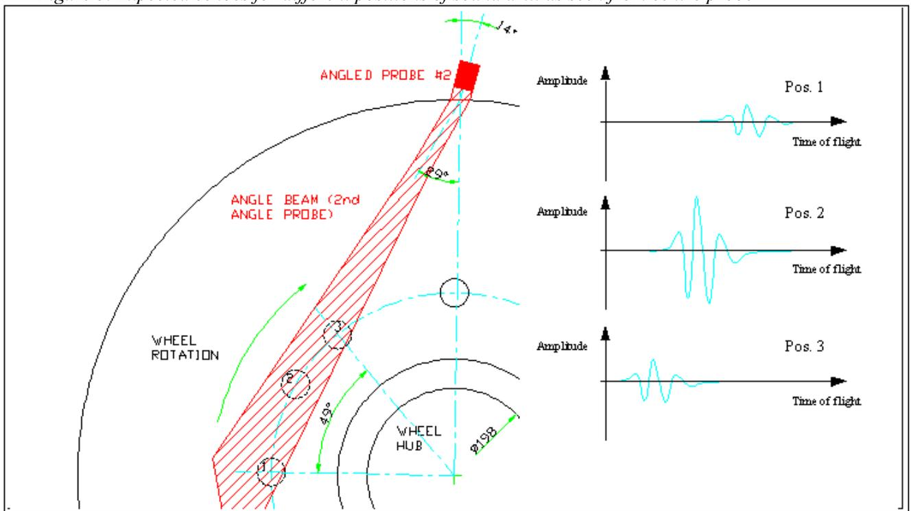
Figure 4. Expected echoes for sound drill as seen from angled probe
