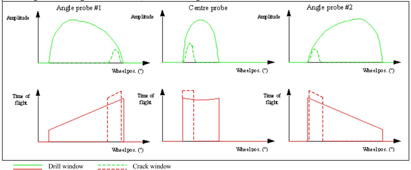
**Figure 8 Enhanced detection of small cracks with double window processing**
