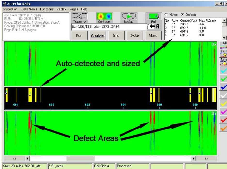
Figure 6. Walking Stick screen layout showing defective rail
