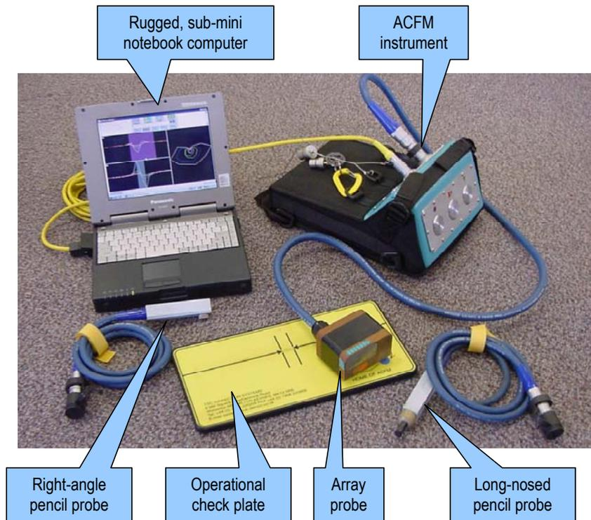
Figure 7. ACFM inspection equipment for Bombardier Transportation
