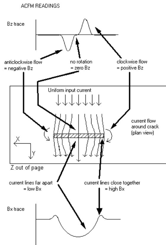
Figure 1. ACFM currents flowing around a defect
