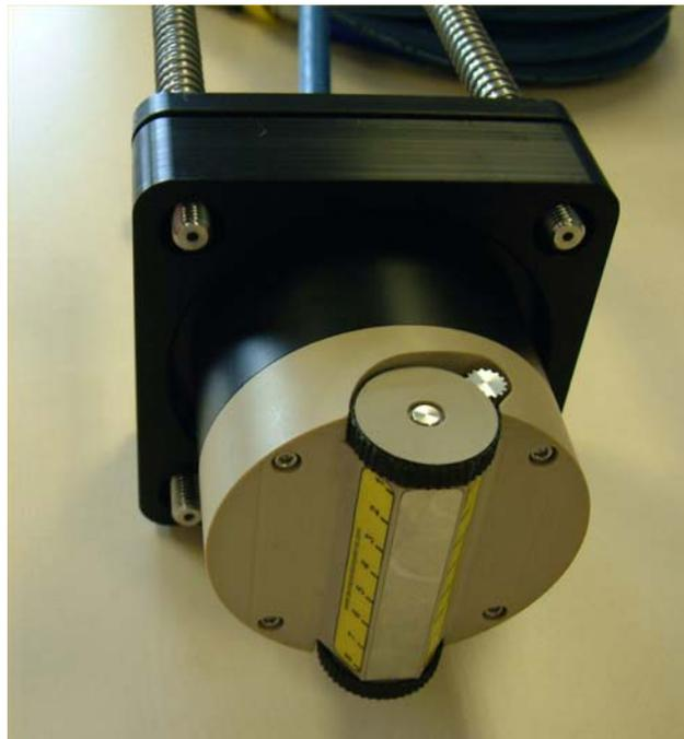
Figure 3. ERB ACFM array probe
