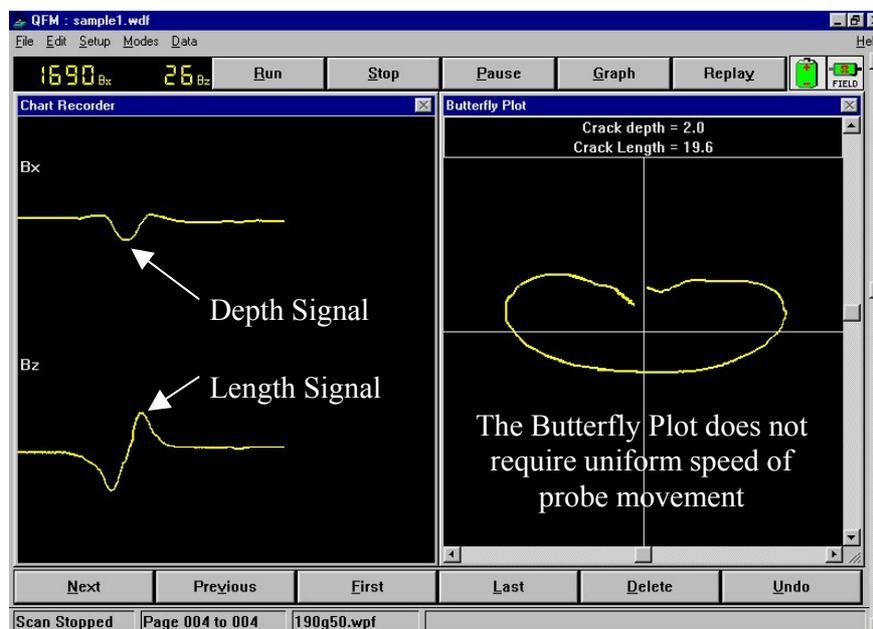
Figure 2. Typical ACFM signal response to a defect
