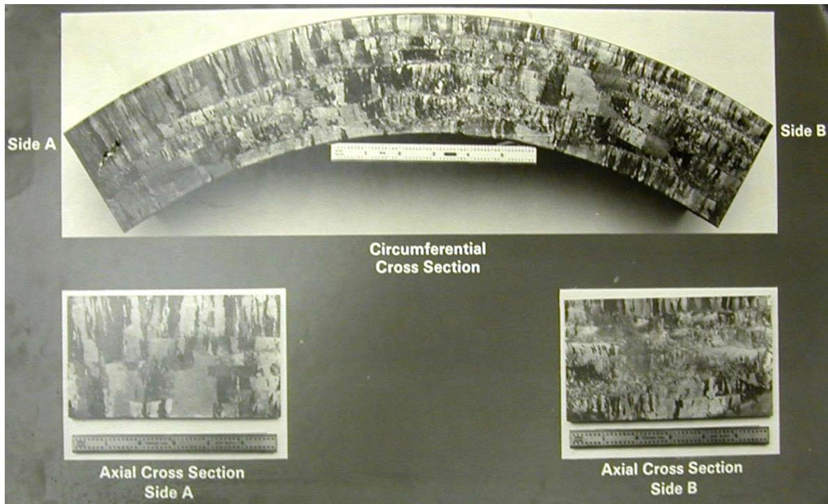
**Figure 1. Circumferential and Axial Cross Sections of Thick-Section, Centrifugally Cast Stainless Steel Pipe, Illustrating a Mixed Columnar-Equiaxed Macrostructure with Multiple Layers and Nonuniform Mixing of Grains**
