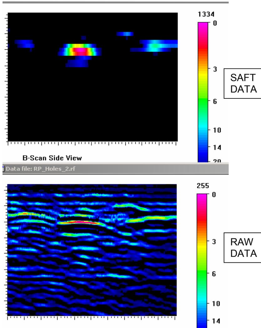
**Figure 4. Visual Illustration of Unprocessed Ultrasonic Data Acquired on a Rail Products & Fabrications, Inc., Frog with Machined Reflectors and the same Raw Data after SAFT Processing. Side Views (left) and Top Views (right).**
