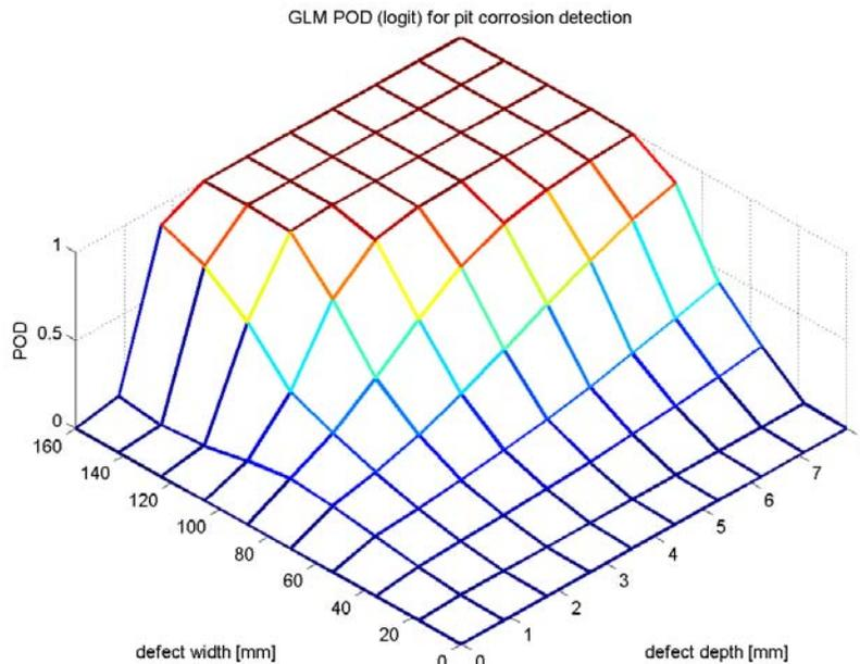
Figure 4: POD-surface as function of defect depth and defect width.
