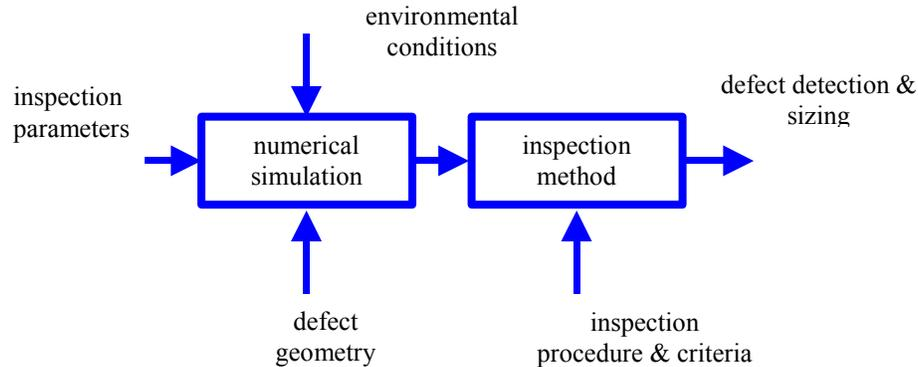
Figure 2: Schematic set-up of the inspection-modeling environment.
