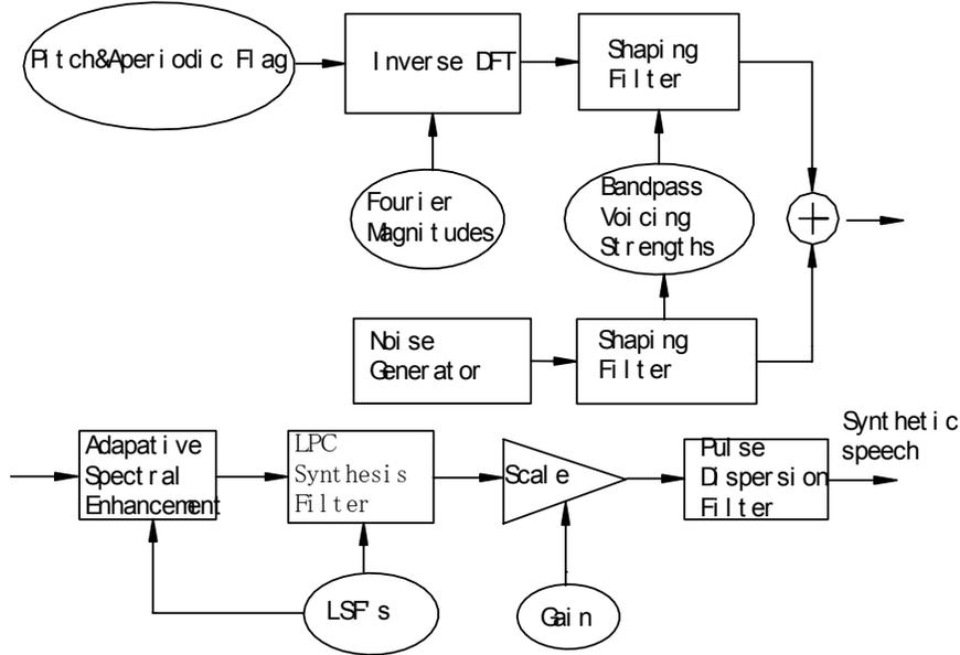
Figure 1. MELP Decoder Block Diagram
