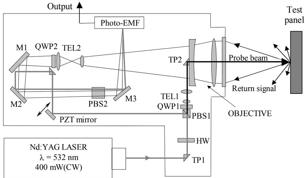
Figure 1 Schematic layout of Lason photo-EMF receiver
