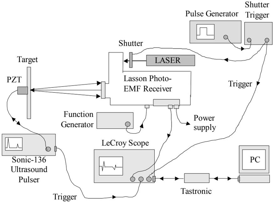
Figure 2 Experimental arrangement
