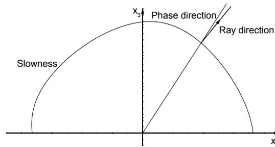
Fig. 6 Diagram of wave traveling in medium 2
