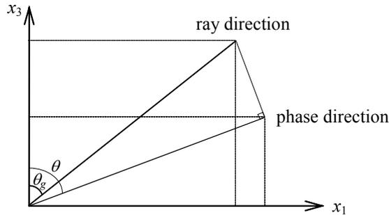
Fig.4 Relationship between ray direction and phase direction
