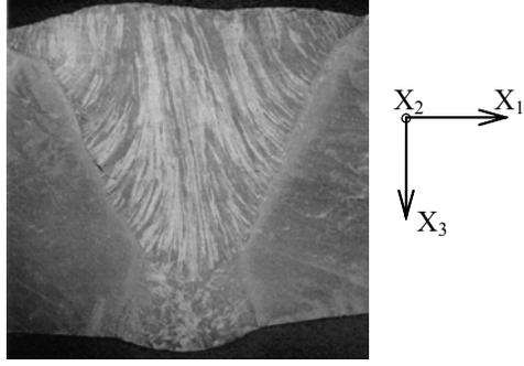
Fig.1 Macrograph of an austenitic stainless steel weld
