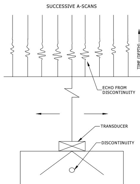
**Figure 1: Data Acquisitions of A-scans in SAFT**
