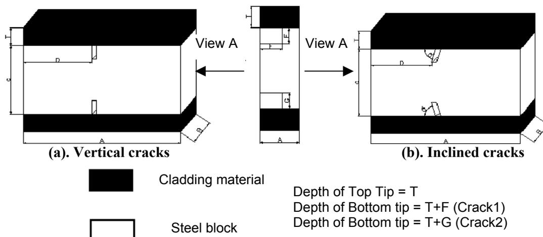
**Figure 4: Schematic diagram of the steel blocks showing the location and size of the sub-cladded vertical and inclined simulated cracks (slits)**
