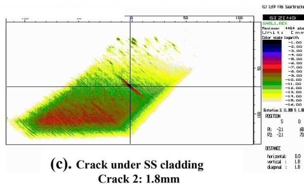
Figure 8(c). SAFT image from inclined simulated crack
