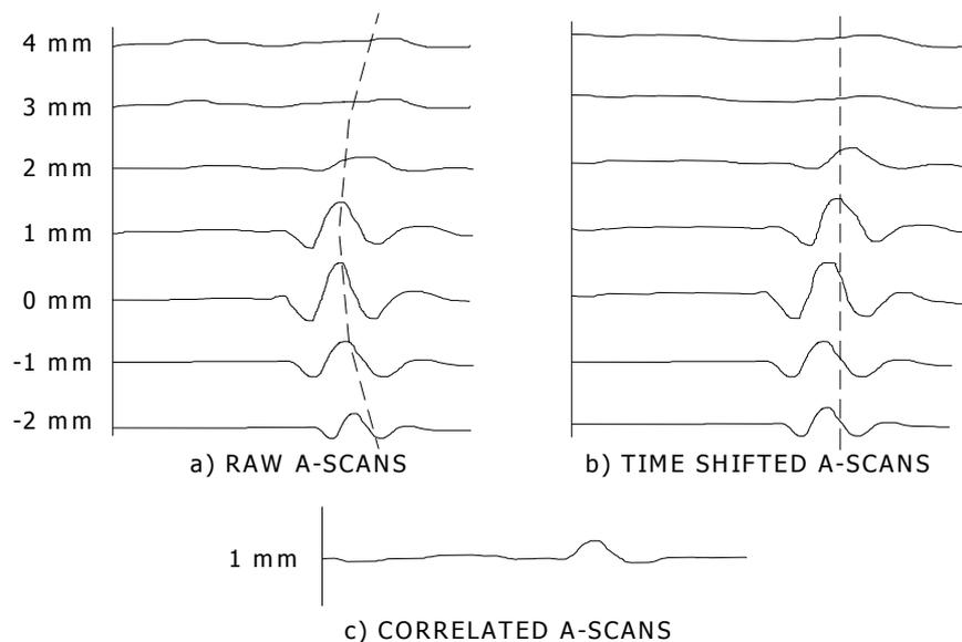
**Figure 3: Showing destructive interference**
