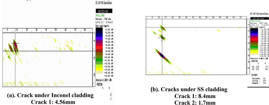
Figure 8 (a) and (b). SAFT images from vertical simulated cracks (slits)
