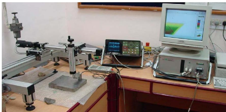
**Figure 5: Experimental set up of SAFT**
